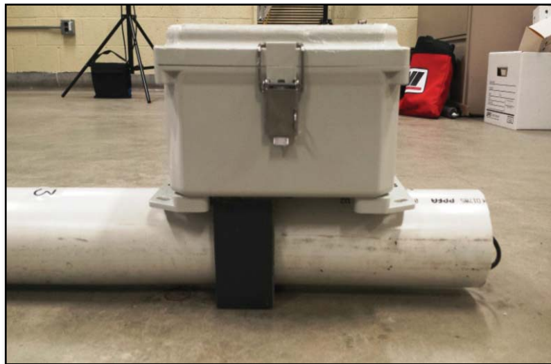
Figure 20. Packaged Smart Scour-sensing Post (Image by Author)
