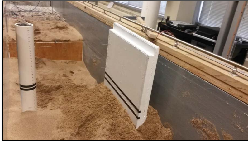
Figure 43. Flume Setup for Pier and Abutment Experiment (Image by Author)
