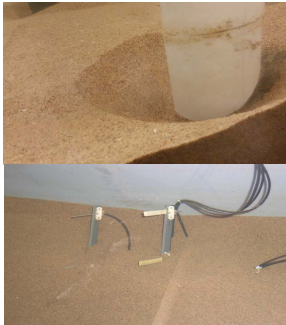
Figure 45. Scour Hole Developed (Image by Author)
