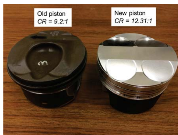
Figure C.1: Stock and new piston top designs [2]
