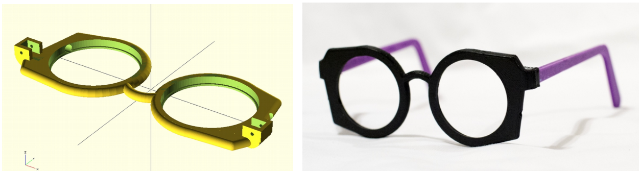
Figure 4. a) 3-D design of self-refractive glasses using the Adspec lenses and first generation syringe system, b) digital photograph of the design which has a customizable component (e.g. color choice of the user).
