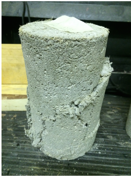
Figure 5.5 Sisal Fiber Cylinder 1 (M3) Compressed Beyond Failure
