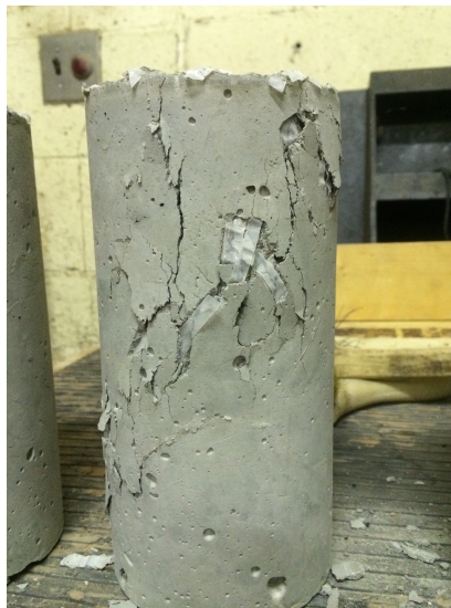
Figure 5.6 PET Plastic Cylinder (M5) Immediately After Failure
