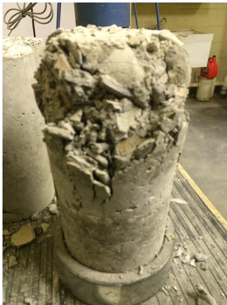
Figure 5.3 Coconut Shell Cylinder (M1) Immediately After Failure
