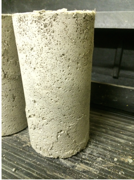
Figure 5.4 Sisal Fiber Cylinder (M3) Immediately After Failure
