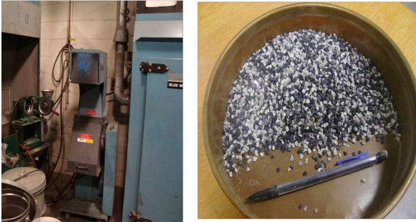
Figure 4.1 Electronic waste materials size reduction equipment, industrial shredder and pulverizer on the left and the source ABS e-waste plastic samples on the right.
