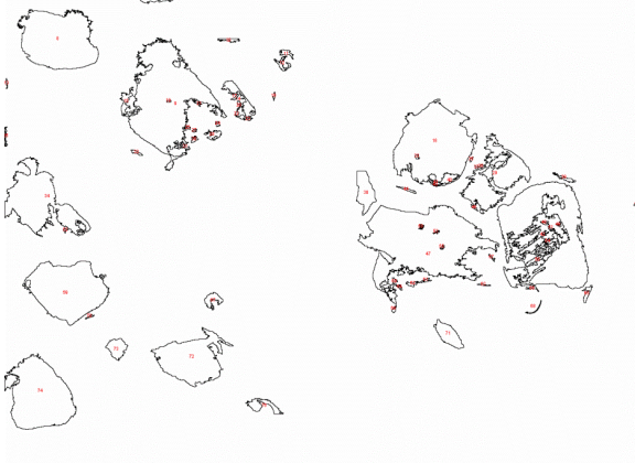
Figure 5.5 ImageJ particle size distribution boundaries of HIPS particles from SEM photograph
