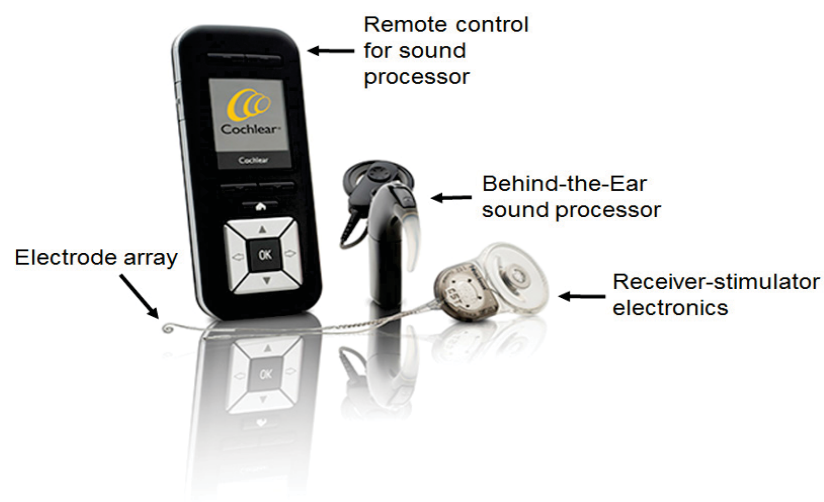
Figure 2.6. Nucleus CI system from Cochlear Limited [31]. Picture provided courtesy of Cochlear Americas, © 2014 Cochlear Americas.
