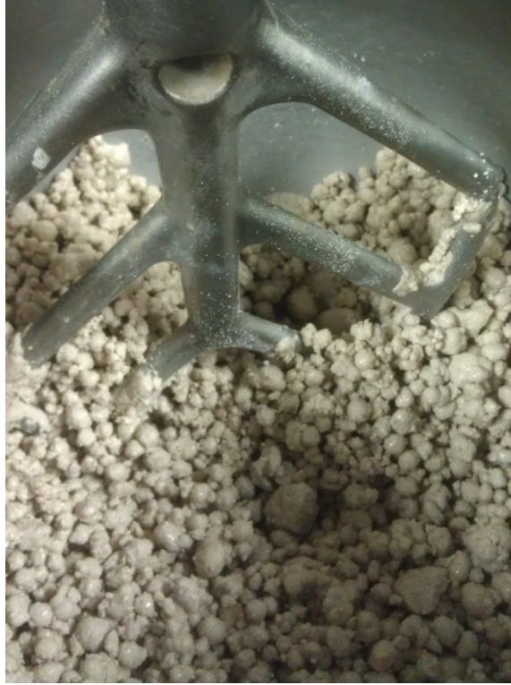
Figure 3.10. Balls formed in mixture with not enough liquid present.
