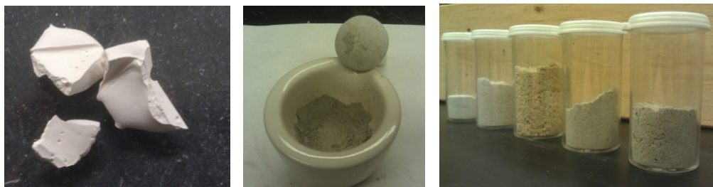
Figure 3.30. Cured paste samples (left), paste sample being crushed by mortar and pestle (center) and various pastes ground into powders in preparation of degree of reaction experiments (right).
