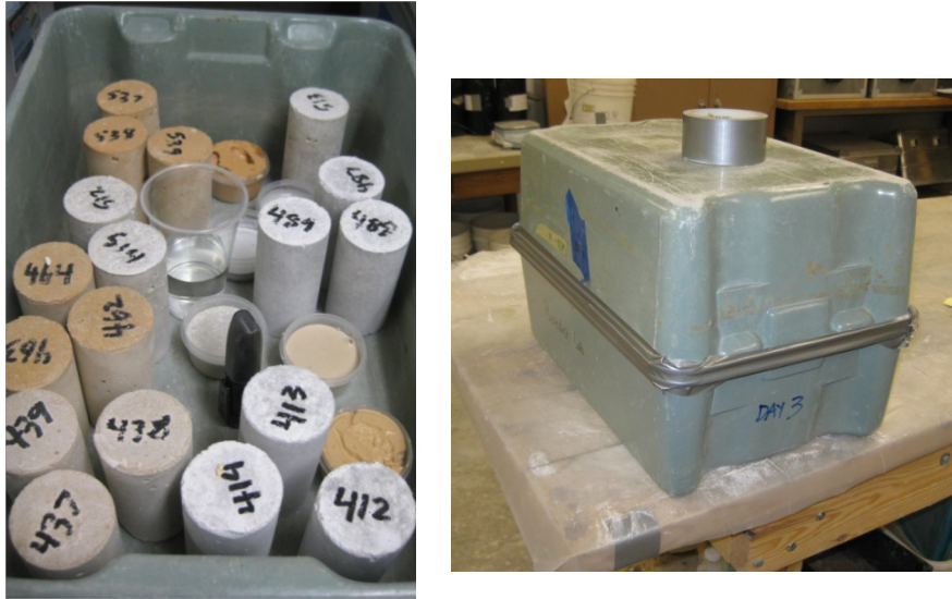
Figure 3.15. Internal (left) and external curing (right) conditions used to maintain desired curing conditions.
