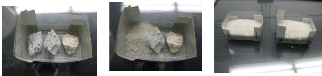
Figure 3.19. Billet boxes filled with samples, then graded Ottawa sand.
