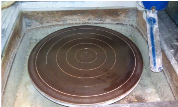
Figure 3.22. Diamond Pacific grinding wheel, used for holding pressure sensitive adhesive backed mineralogical papers.
