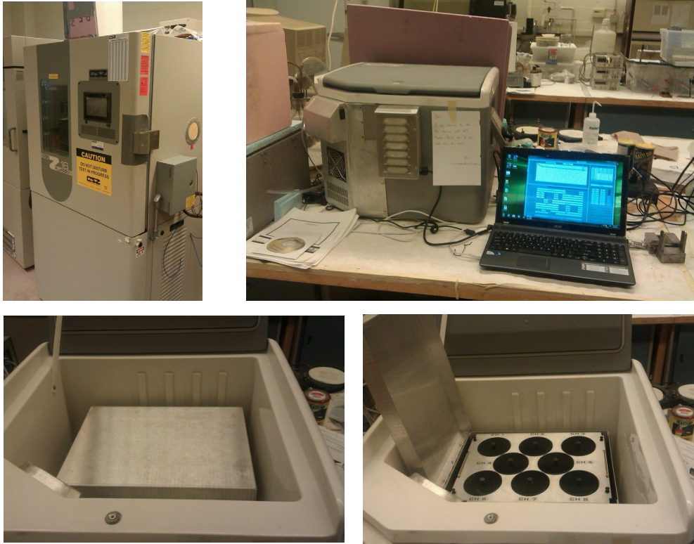
Figure 3.34. Isothermal calorimeter at University of Toronto.
