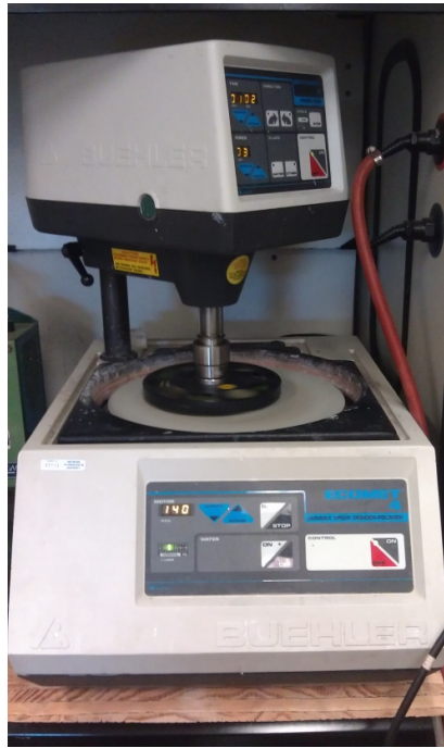
Figure 3.23. Beuhler Isomet used to do the finer polishing with diamond paste media on nylon cloths.
