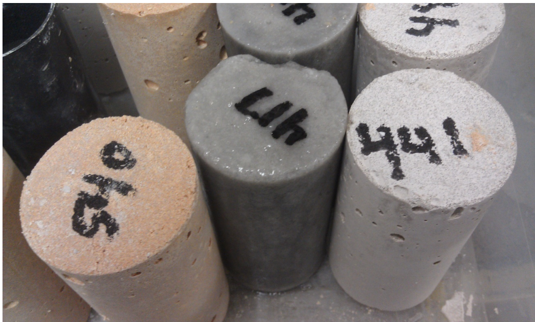
Figure 4.53. A depiction of how wet the low-Al glass was even after 14 days of curing as compared to the other mixtures.
