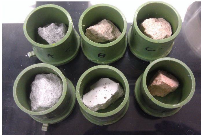
Figure 3.18. Circular sample molds filled with samples prior to vacuum impregnation.
