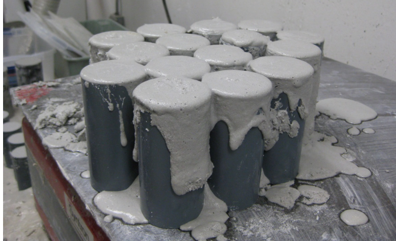
Figure 3.14. Molds after vibration on vibration table.
