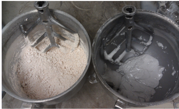
Figure 3.11. Visible difference in water demand for 100% metakaolin (left) and 100% glass (right) activated with the same amount of activator, water and source material by mass.
