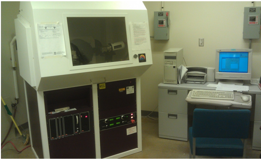
Figure 3.26. Powder X-ray diffraction (XRD) machine.
