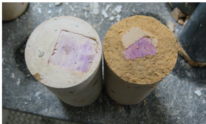
Figure 3.16. Specimen damage during demolding in samples containing metakaolin.
