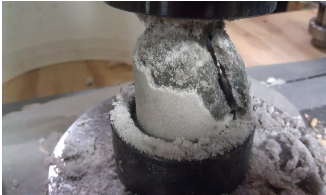
Figure 4.55. 100LA mixture after compression testing showing color differences between interior and exterior of cylinder at 14 days. The interior still appeared and felt damp and slimy despite being very dense.
