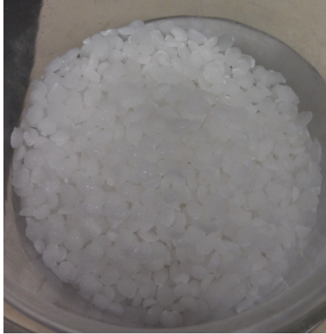
Figure 3.7. NaOH flake pellets prior to solution preparation.
