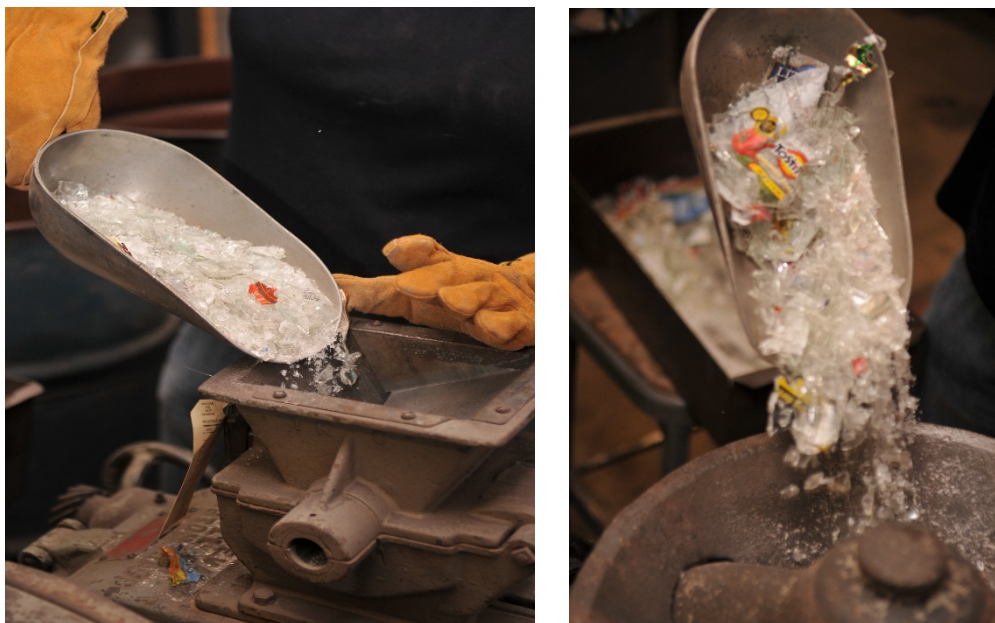
Figure 3.1. Waste packaging glass being crushed in a jaw crusher (left) and a gyratory crusher (right). Wrappers, cap rings, etc. are quite easy to remove by sieving once the glass gets down to a certain size.
