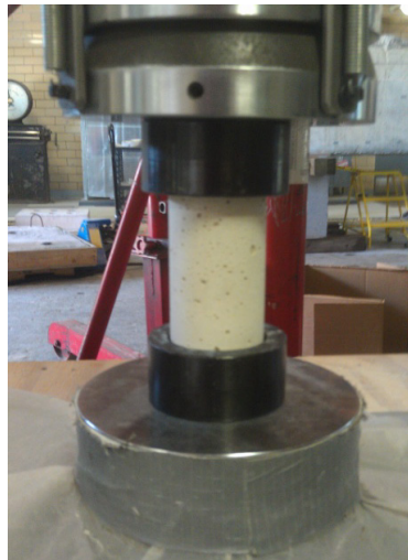
Figure 3.35. Compressive strength testing set up on the Material Testing System (MTS) machine.
