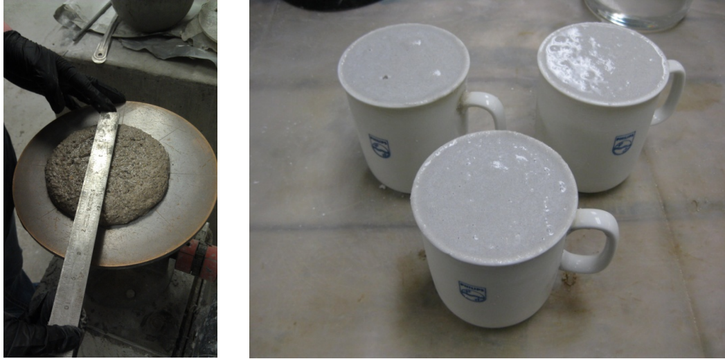
Figure 3.13. Flow table test (left) and unit weight setup (right).
