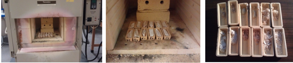
Figure 3.32 Degree of reaction tests following calcination in muffle furnace.
