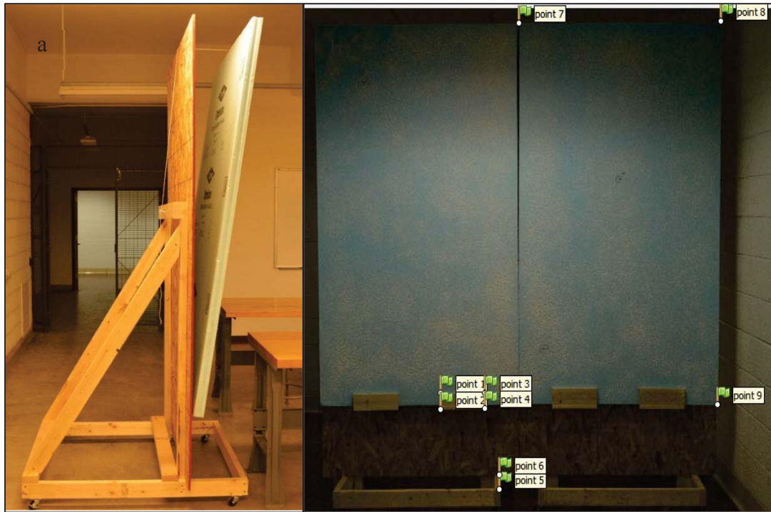
Figure 2-4 Retaining walls small scale model. (a) Single unit structure with the panel rotated about a bottom hinge to simulate deflection. (b) Scaled model consisting of two units to simulate two sections of retaining wall meeting at an expansion joint.
