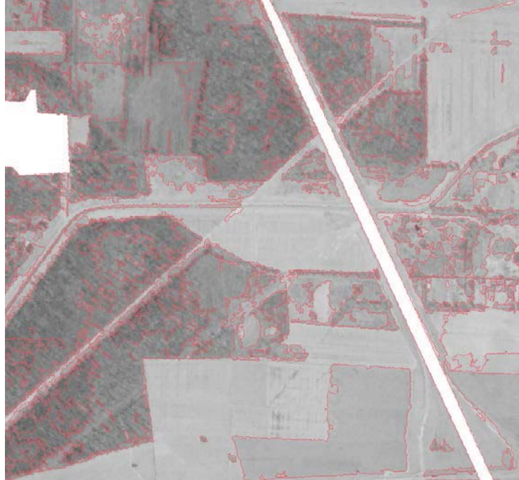
Figure 3.7: Image segmentation utilizing SPRING for Pond Creek Watershed, KY (USGS station 03302000). Red lines are segmented area boundaries.
