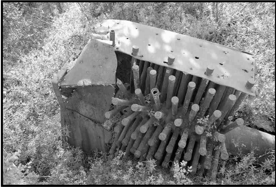
Figure 5.7: Porcupine boiler (Goddard 2010)
