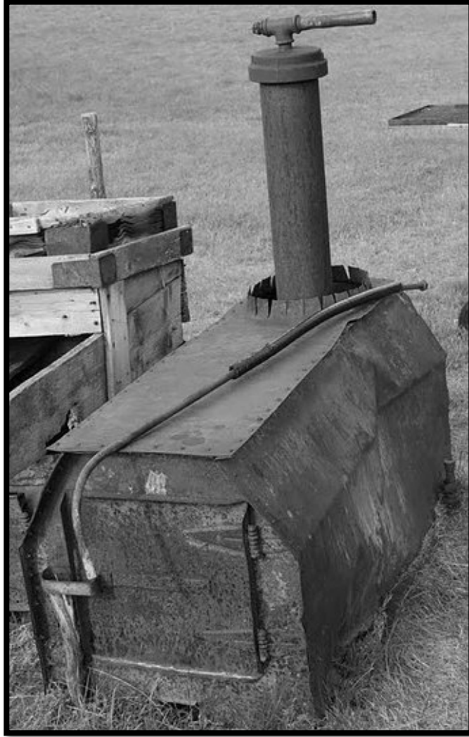
Figure 5.8: Doghouse boiler (Goddard 2010)
