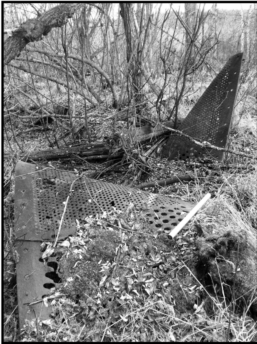
Figure 6.21: Damaged trommel screens (Baeten: 2011)
