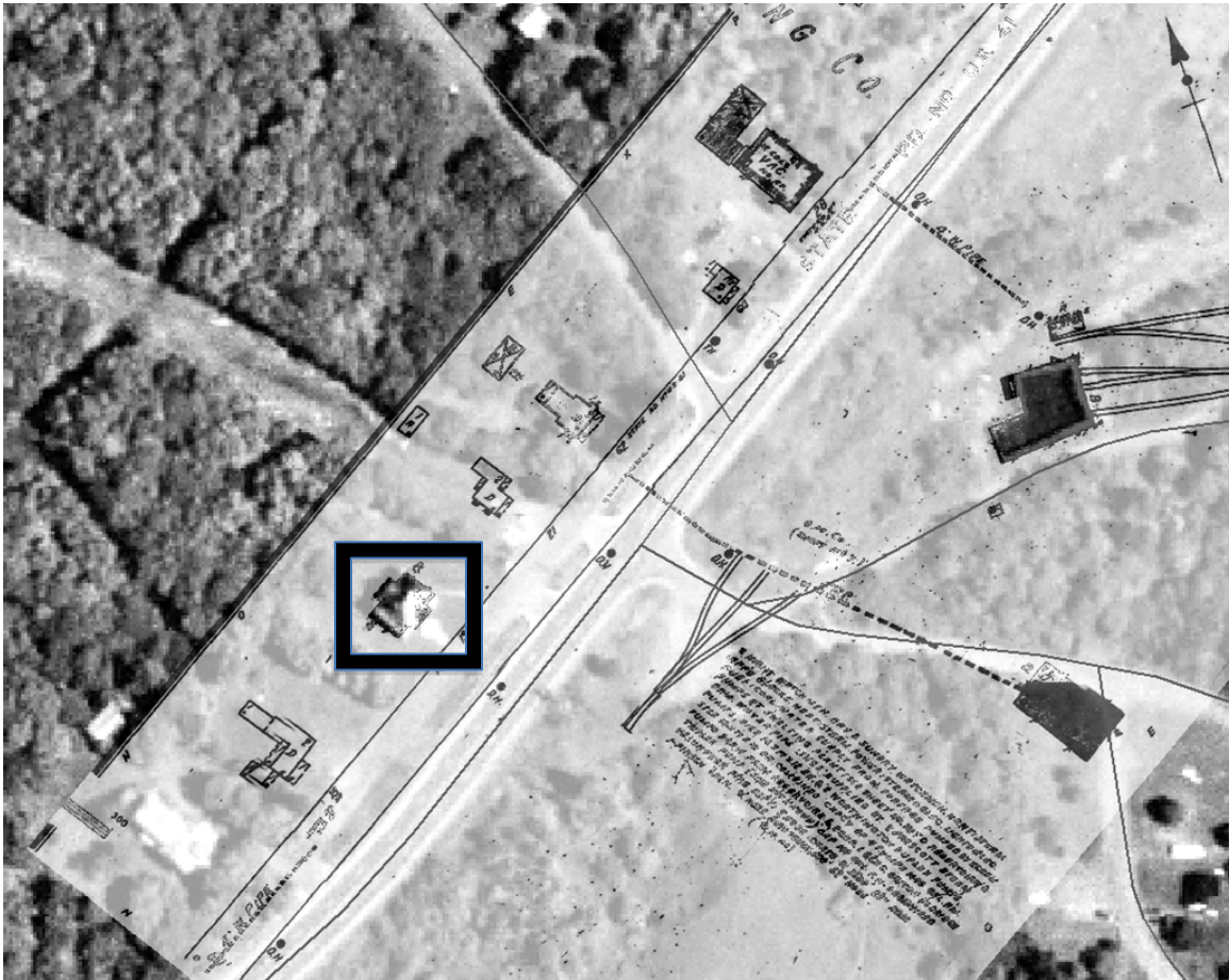
Figure 5.1: 1928 Sanborn map with georeferenced structures. These structures will create the basis for digitizing the polygons that will be used in ArcScene. The location of the office is outlined by the black box. Created in ArcMap by author.
