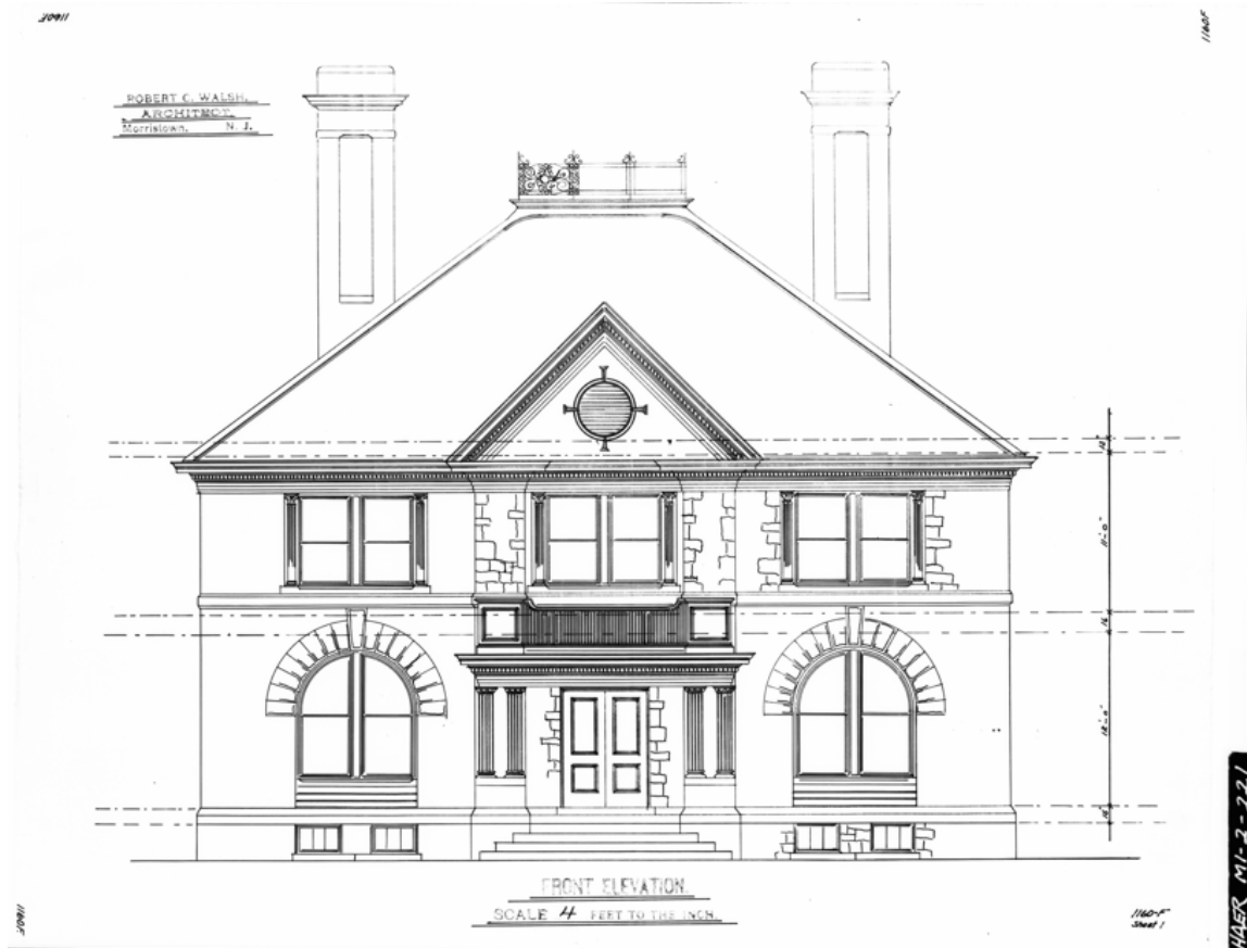
Figure 4.7: Original front elevation drawing for QMC office by architect Robert C. Walsh. The major difference between the drawing and actual construction was the change in shape of the dormer window. Photograph courtesy of Library of Congress, HAER Documentation, Quincy Mining Company.
