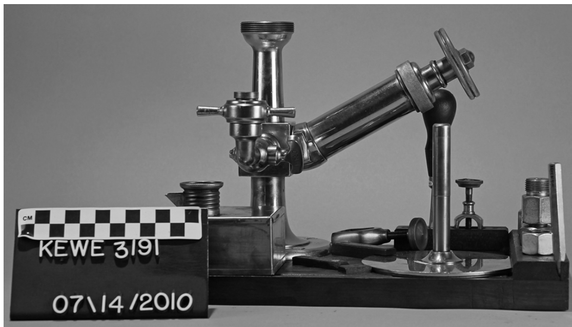
Figure 5.12: Example of a QMC office object. This is a dead weight steam pressure gauge tester. A pressure gauge would be attached and weights would be added to determine if the pressure gauge was working properly. Image courtesy of KNHP, 2010.
