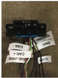
Figure 2.21: OBDII connector wiring (photo by author).
