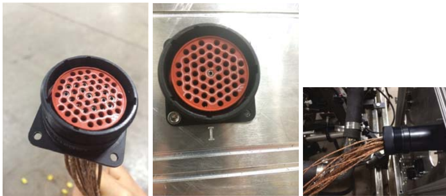
Figure 2.22: Thermocouple wiring (photo by author).
