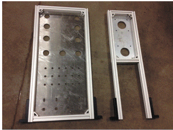
Figure 2.5: Manufactured interface panels (photo by author).
