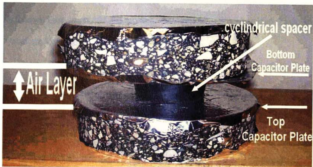
Figure 5.8: Setup for asphalt samples for calculating air dielectric in TDR experiment
