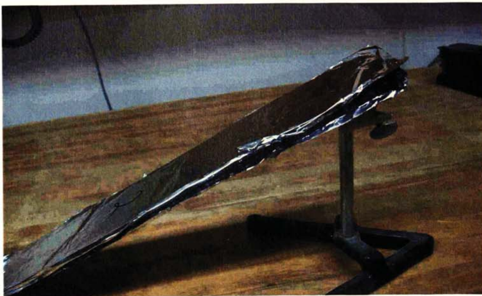
Figure 5.5: Thin rectangular pavement sample used in TDR experiment
