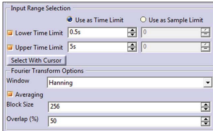
Figure 65: Processing variables used to calculate the FRFs in the DSP Case
