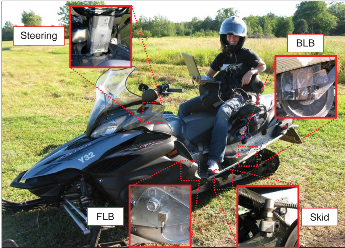
Figure 15: Operational test setup including response measurement locations with respect to the body of the sled
