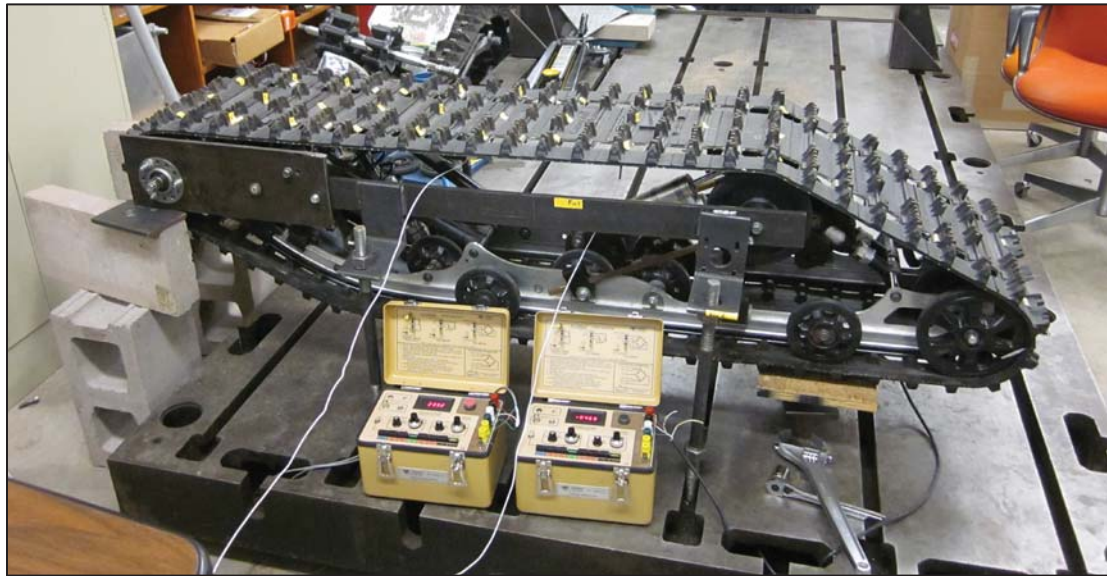
Figure 35: Rear suspension test set up for track modal analysis
