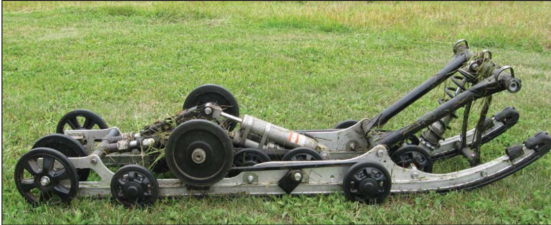
Figure 27: Suspension A, the baseline rear suspension configuration
