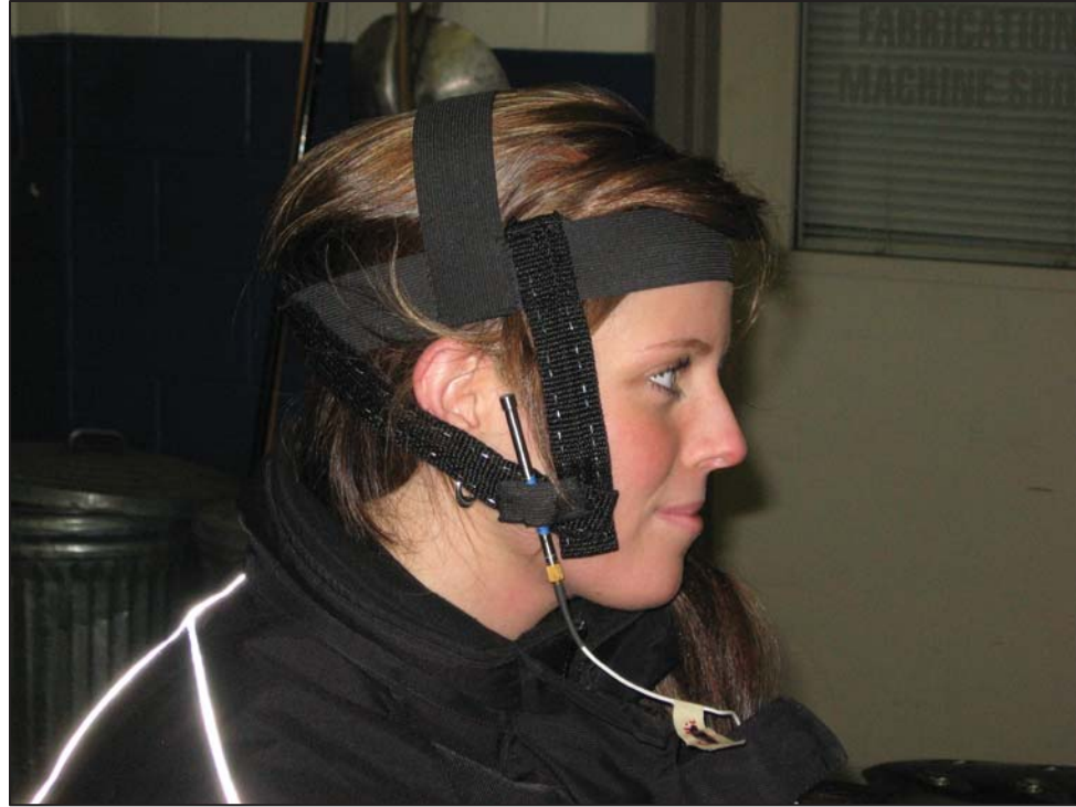
Figure 13: Custom harness designed to hold a 1/4" microphone 1" from the operator's right ear inside a snowmobile helmet
