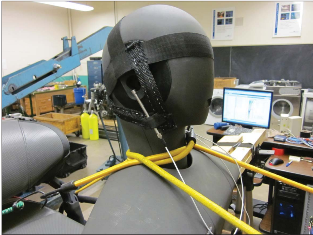
Figure 39: The Aachen head fitted with a custom microphone harness for the impedance measurements
