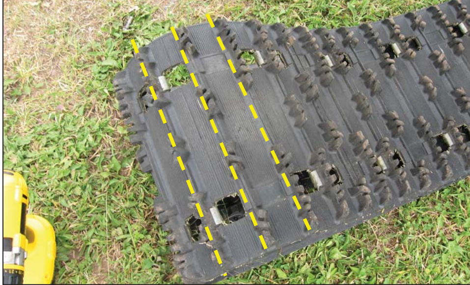
Figure 5: Picture of the snowmobile track identifying three of the fiberglass stiffener rods molding under the rubber in the track by the yellow dotted lines
