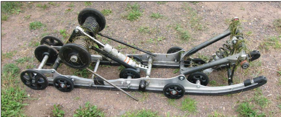
Figure 28: Suspension B, same suspension as A with two less guide wheels
