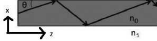
Figure 1: Geometrical optics ray propagation.
