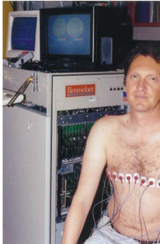
Figure 1-3 Electrical Impedance Tomography Device with electrodes attached to a patient's chest. Taken from Cheney, Margaret, David Isaacson, and Jonathan C. Newell. "Electrical impedance tomography." SIAM review 41.1 (1999): 85-101 Copyright ©1999 Society for Industrial and Applied Mathematics. Reprinted with permission. All rights reserved. See Appendix A for documented permission
