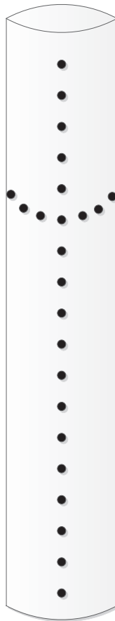
Figure 3-1 Diagram of original test apparatus showing electrode locations
