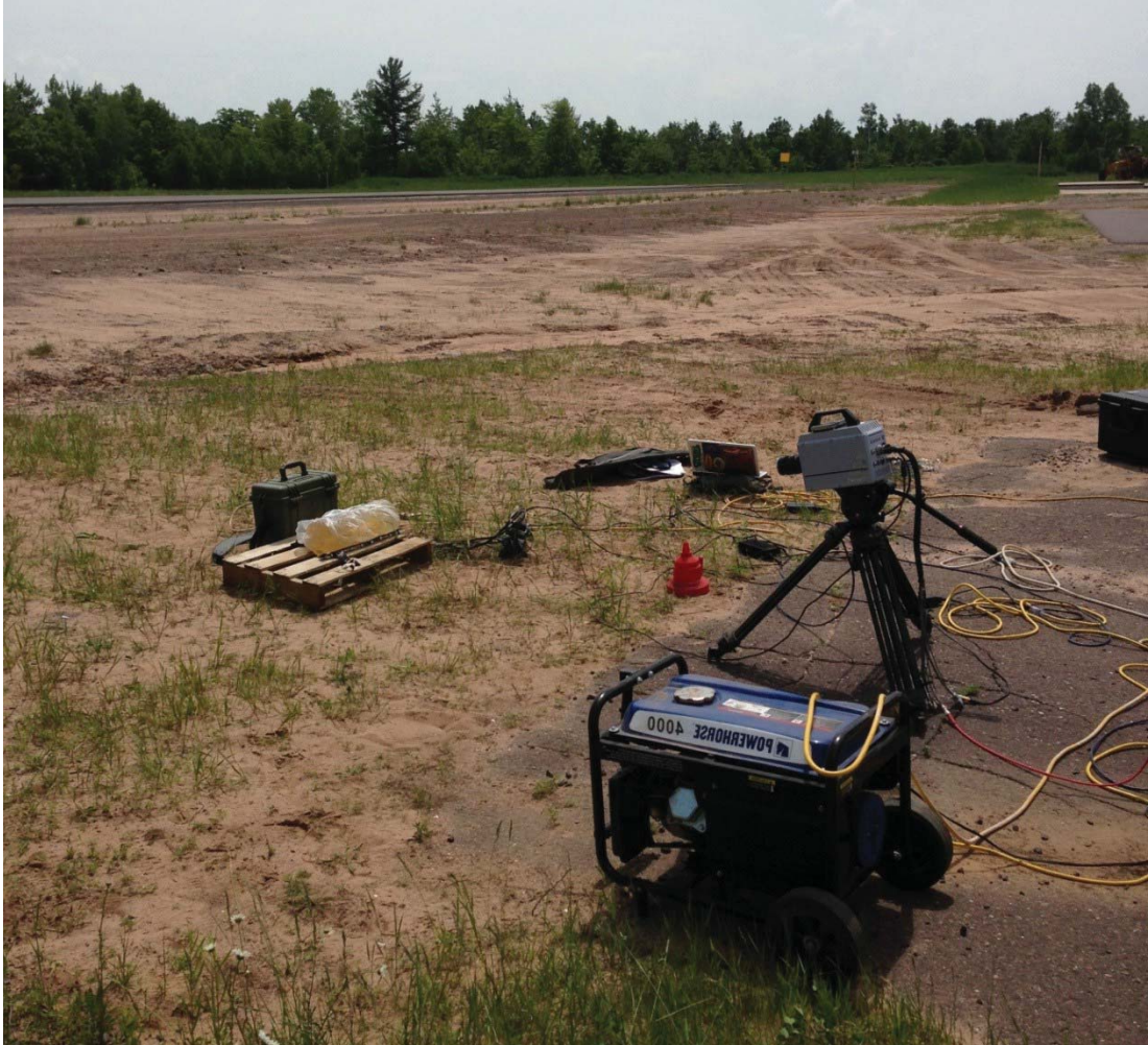
Figure 3-21 Test setup for temporary cavity imaging
