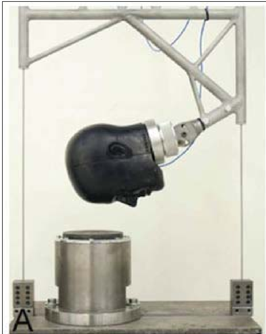
Figure 2.2 NOCSAE Drop Test: Photograph of Experimental Setup similar to that in MTU, MEEM Biomechanics Lab
