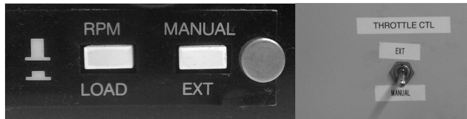
Figure 3.13: Switches used for switching between manual control mode and external voltage control mode
