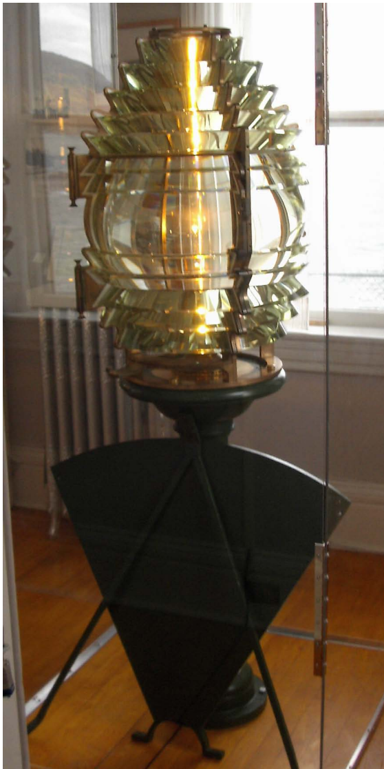
Figure II.5: Photograph of the third order Fresnel lens on display at the Eagle Harbor Lighthouse museum. (Lisa Gillis, October 11, 2009)
