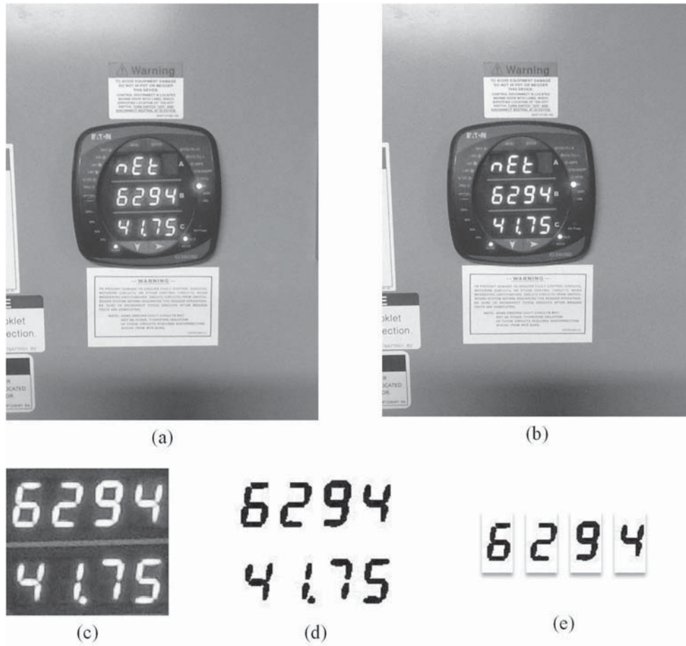
Figure 3.10: Digital Images Preprocessing and Image Segmentation in 5 Steps: (a) Original Image. (b) Grayscale Image. (c) Binarization Outcome. (d) Counter-color Outcome. (e) Analyzable Objects.
