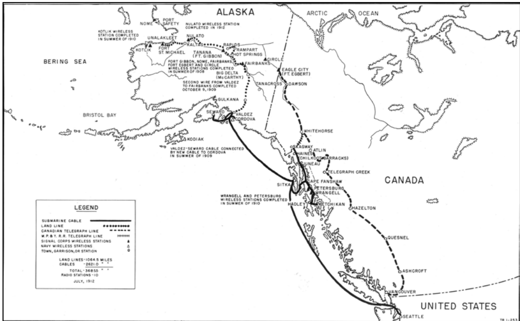
Figure 6: Communication lines installed by 1912 (CECOM Historical Office, Image 4158f). 161
