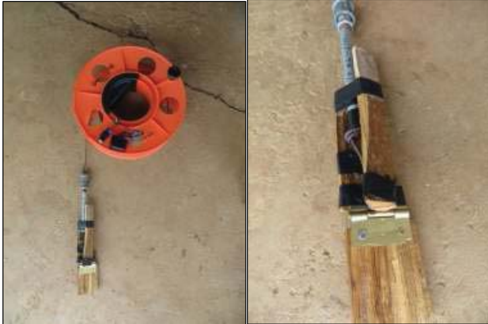
Figure 17: Homemade water level sounder with detail of the circuit connection
