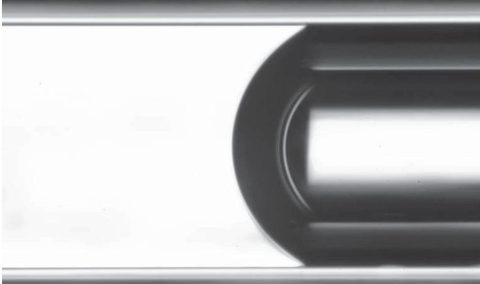
Figure 5.1. Image of gas-liquid interface of a liquid plug in a microchannel. The interface acts as a lens that bends the light away from the optical path creating the dark region near the meniscus.
