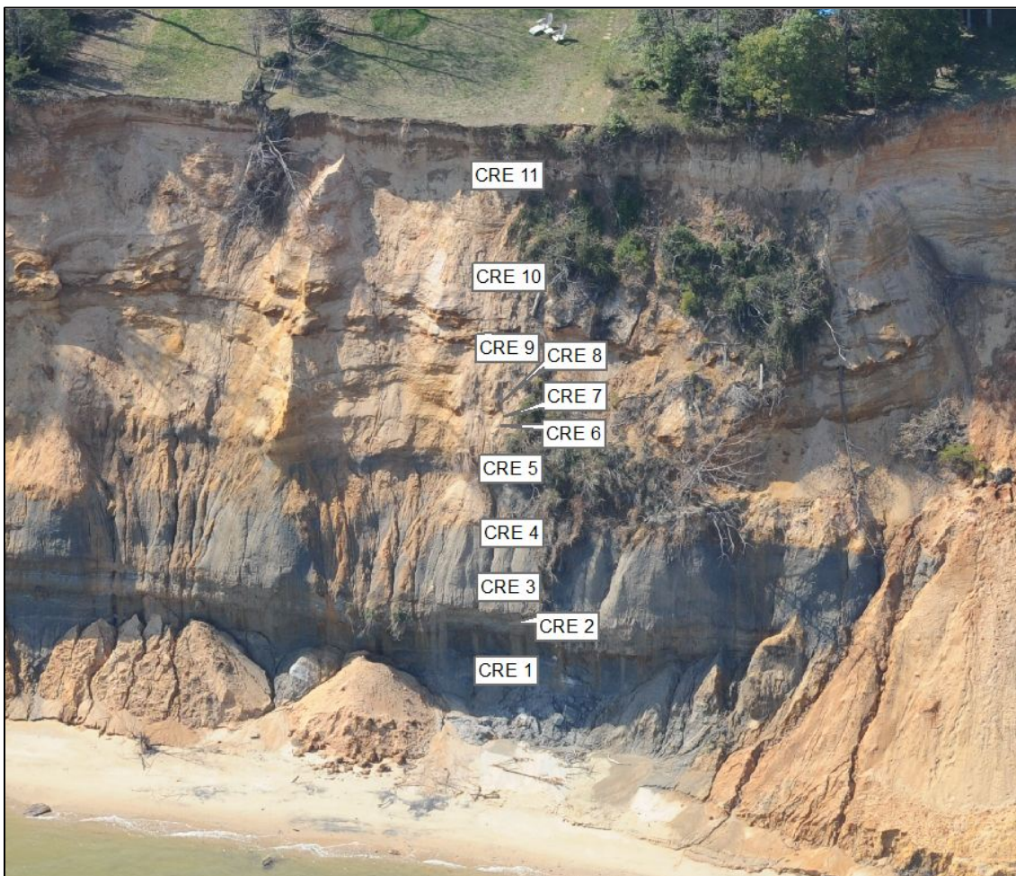
Figure 7: Soil Layers Identified for CRE2 in Order for Soil Layer Thicknesses to be Calculated (image data source: Calvert County Government 2012)
