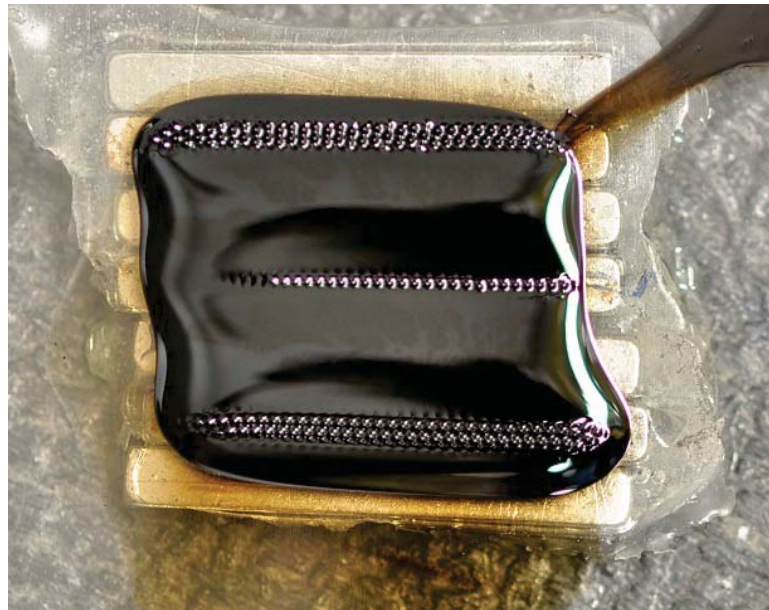
Figure 5.5: Image of ferrofluid on a linear Halbach array. The length of each individual magnet was 25.4 mm.
