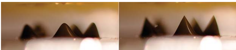
Figure 4.10: EMIM-NTf2 based ILFF in annular fluid holder. Left: ILFF exposed to magnetic field only (Rosensweig instability). Right: ILFF exposed to magnetic and electric field, applied voltage was 2700 V, and emitting ions.
