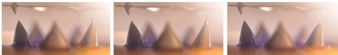
Figure 4.17: Sequence of images elapsed over the course of less than 5 seconds with a constant voltage applied. In the left image, the peak on the right was emitting. In the middle image, the peak grew a long protrusion while still appearing to be emitting. The rightmost image the protrusion “exploded” and appeared to form a cone of spray. The applied voltage was -2750\text{ V} and biased negatively (emitting anions) and the collected current was between 150 and 225\ \mu\text{A} . In all the images there was a downward-facing cone attached to the extraction electrode. This downward-facing cone was created because part of the spray being intercepted by the extraction electrode. After enough ILFF built up on the extraction electrode, the downward-facing cone appeared. It was unknown if this downward-facing cone was spraying toward the lower pool of ILFF.
