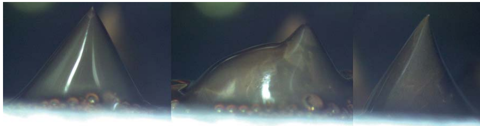
Figure 4.8: Series of images showing a peak emitting, become damaged, and then self-repair and begin emitting again, with no operator intervention. Left: Peak emitting ions, small bubbles visible at the base of the peak. Center: A large bubble appears in the peak, and emission from this peak ceases. Right: After the bubble burst, peak begins emitting ions again.
