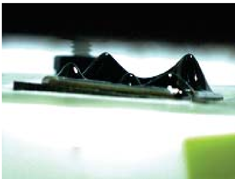
Figure C.7: ILFF (EAN with Sirtex magnetic nanoparticles) with a magnetic field of 297.1 Gauss and applied voltage of -4500 V.)
