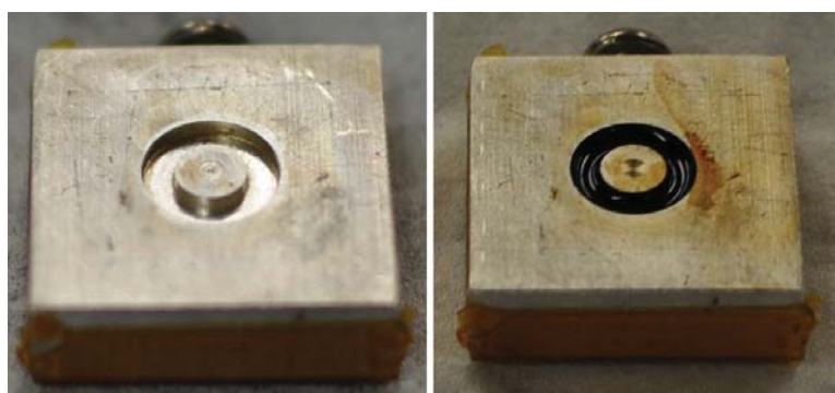
Figure 4.2: Image of aluminum fluid holder. Left: Without ILFF. Right: Trench filled with ILFF.
