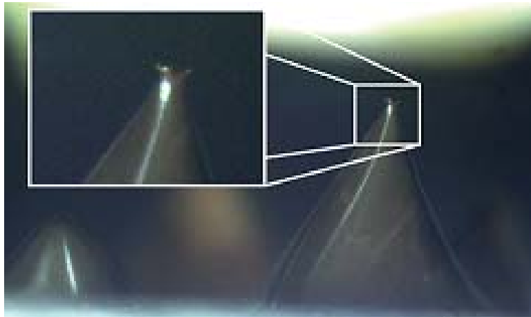
Figure D.8: A zoomed-in image of Figure D.7, with an additional insert focusing on the three emission sites at the tip.
