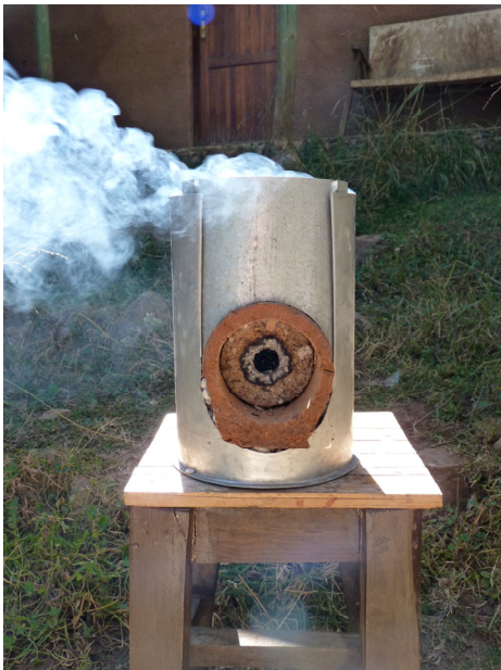
Figure 5.5: Left, preliminary burn test. Right, water-boiling test. (Photos by Brian Barbre)
