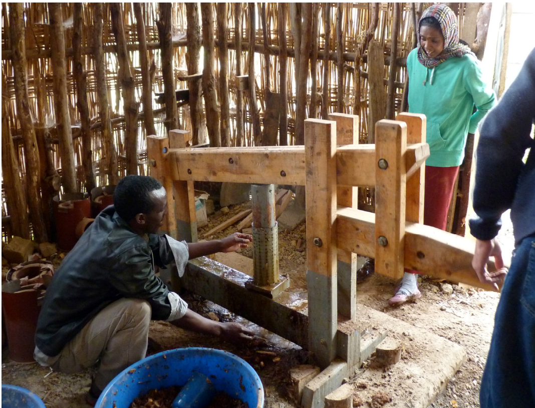
Figure 5.1: Briquette press in use during a training session. (Photo by Brian Barbre)
