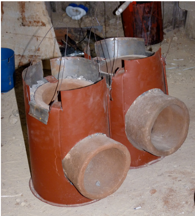
Figure 5.7: Top, stove cross section. Bottom shows two assembled stoves. (Photo and Figure by Brian Barbre)
