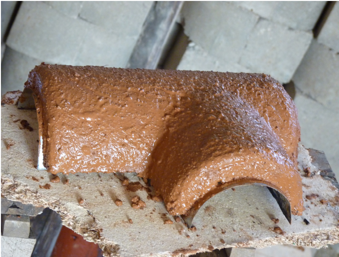
Figure 5.10: Wet ceramic from the mold resting on metal liner. (Photo by Brain Barbre)
