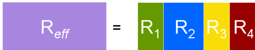
Figure 4.1 - Approximating armor thermal response using an effective resistance
