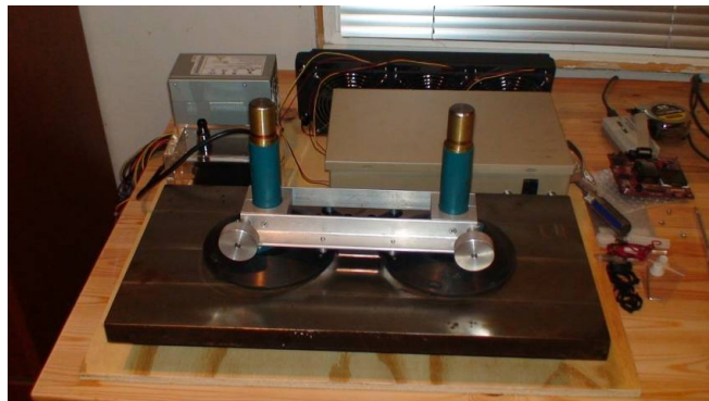
Figure 5.15 - Testing of a homogenous steel sheet (1'x2'x1")
