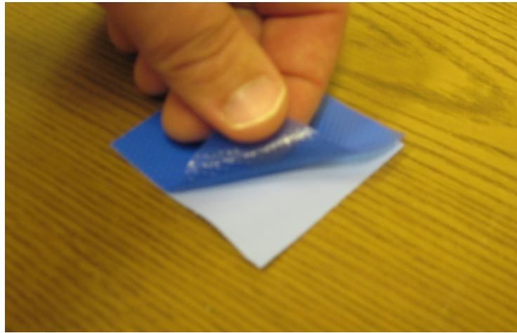
Figure 5.6 - Example of a peel-and-stick thermal interface pad
