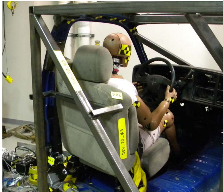
Figure 5.2. Tracking points for dynamic analysis
