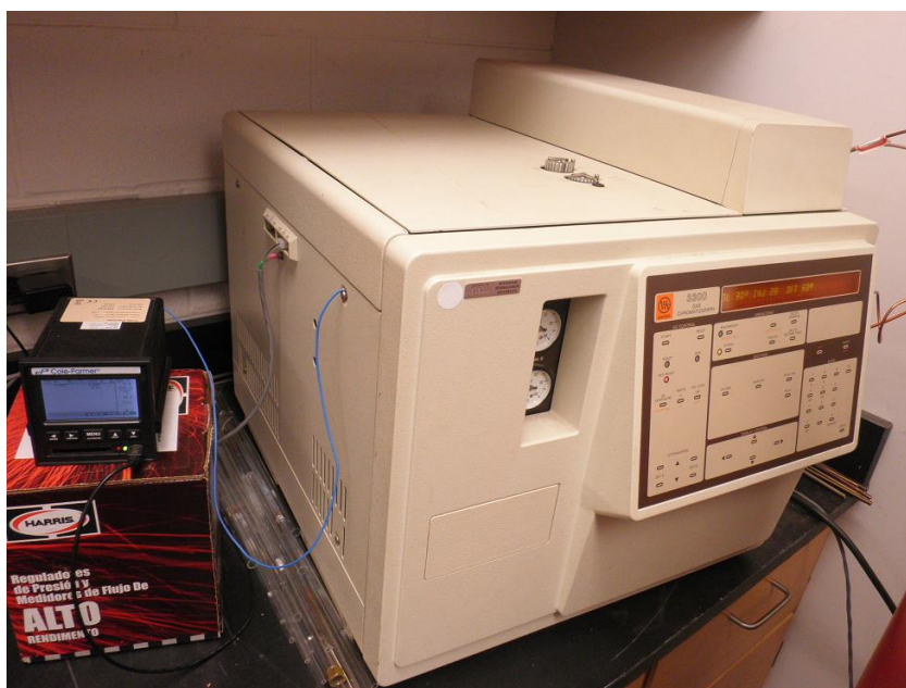
Figure 2.1 Thermal conductivity detector of Varian 3300 Gas Chromatograph.
