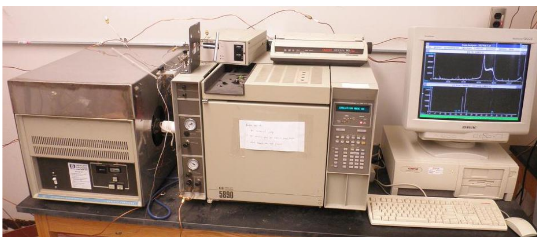
Figure 2.2 HP 5970 series mass selective detector.
