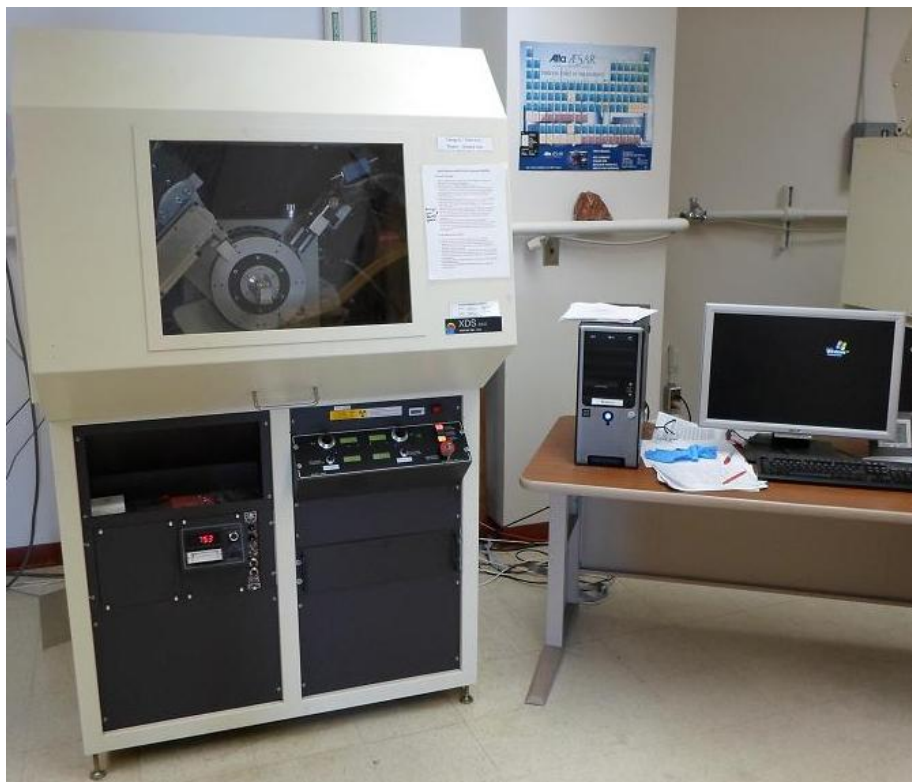
Figure 2.3 Scintag XDS2000 Powder Diffractometer.
