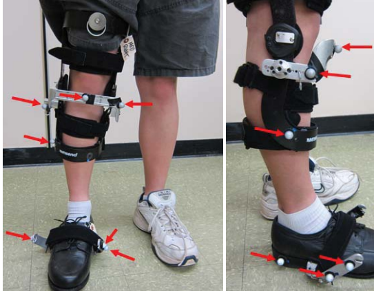
Figure 9. Knee brace and shoe with reflectors. The arrows point to the visible reflectors.
