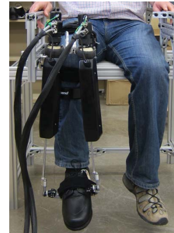
Figure 2. Anklebot mounted to the chair for testing the mechanical impedance in the medial/lateral rotation
