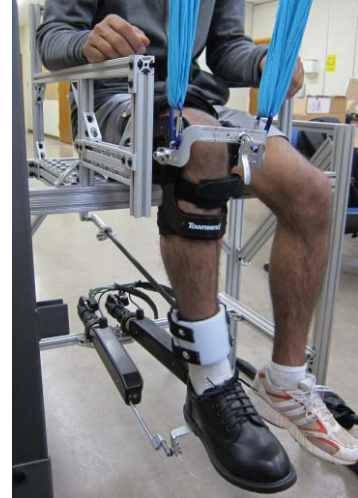
Figure 1. Anklebot mounted to the chair for testing the mechanical impedance in the medial/lateral rotation
