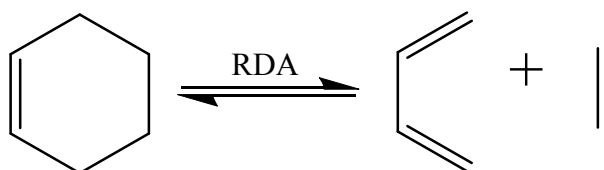
Figure 3.2: Reverse Diels-Alder mechanism
