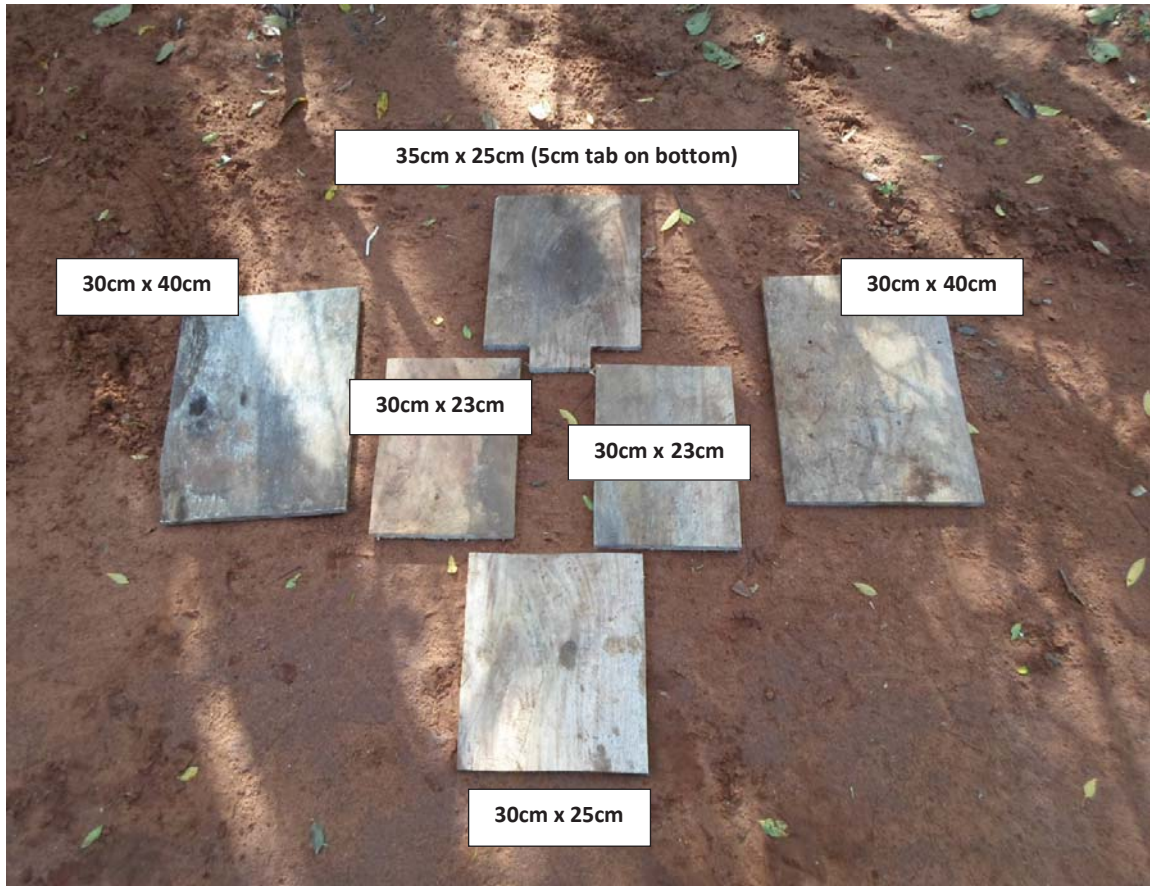
Figure 80: Board sizes and quantities needed for seat construction. Photo by author.
