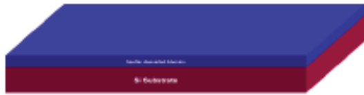
Step 2. Sputter Deposition of 350nm thick Al 2 O 3 layer
