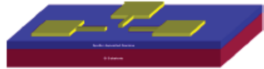
Step 5. Electrode trimming and gap formation using FIB etching technique.
