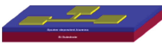
Step 3. Sputter Deposition of 100nm thick Cr layer
