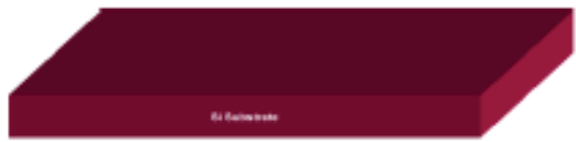
Step 1. Dicing Si wafer to size 5X5mm
