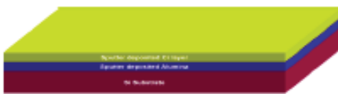
Step 3. Sputter Deposition of 100nm thick Cr layer
