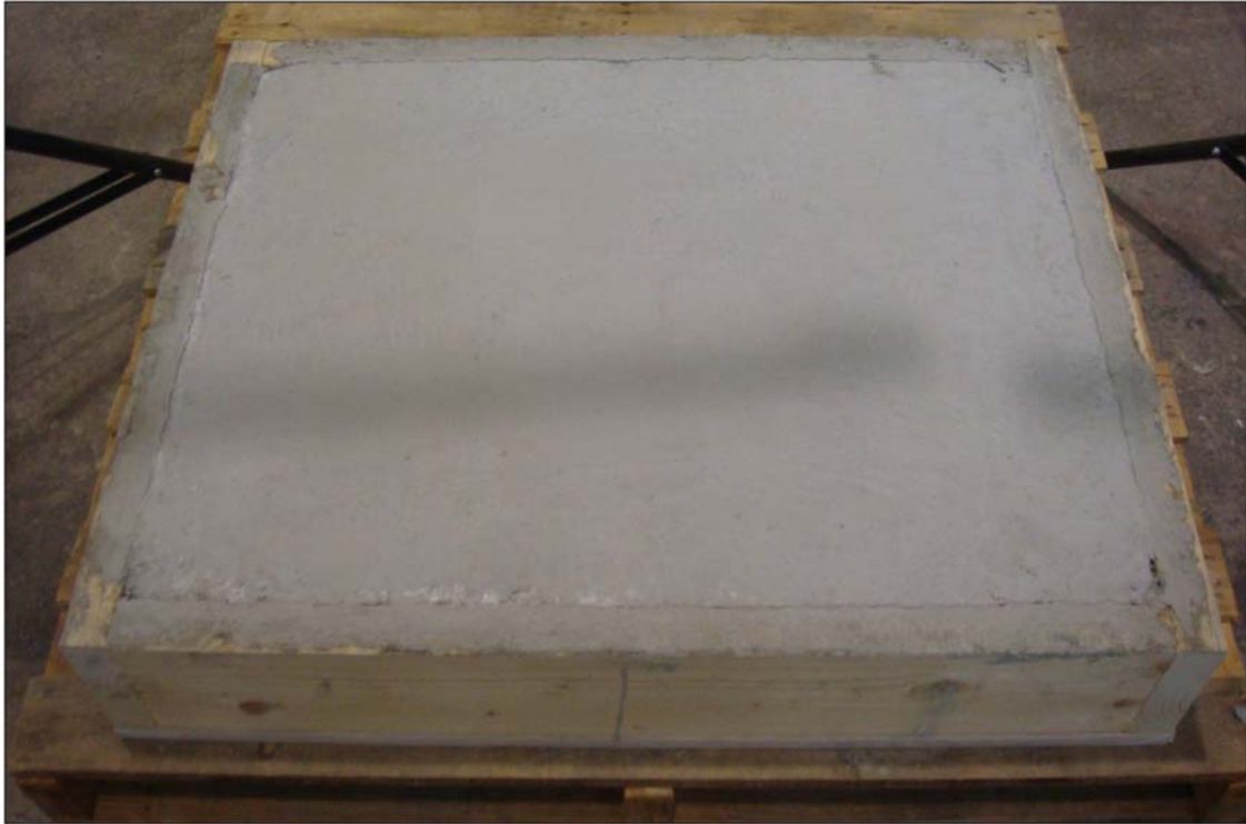
Figure 5.8 Concrete Slab IV after it was built and cured.
