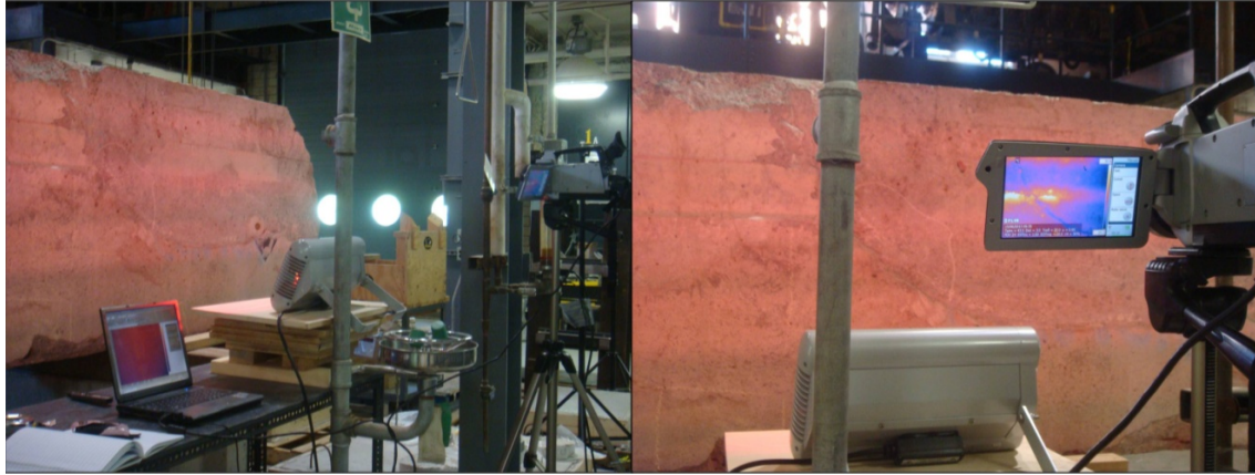
Figure C.4 Active infrared thermography test set-up at the location E1.
