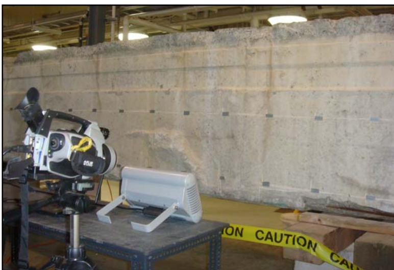
Figure C.3 Active infrared thermography test set-up at location W3.
