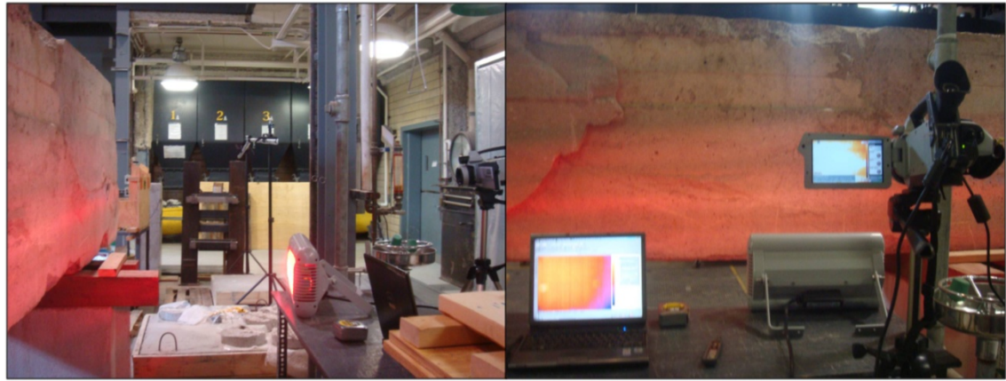
Figure C.5 Active infrared thermography test set-up at the location E2.
