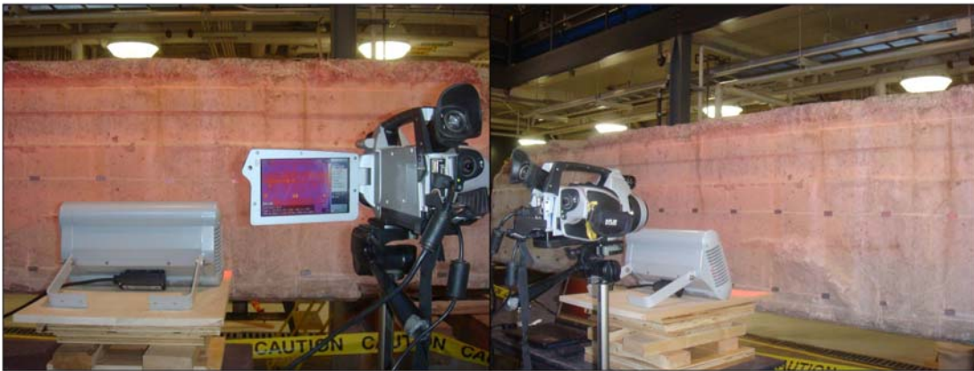
Figure C.2 Active infrared thermography test set-up at the location W2.
