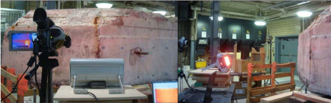
Figure C.1 Active infrared thermography test set-up at the location W1.
