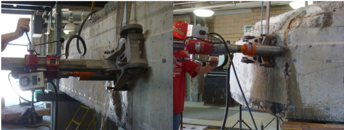
Figure 6.43 Coring procedure on the Silverbell Bridge beam.
