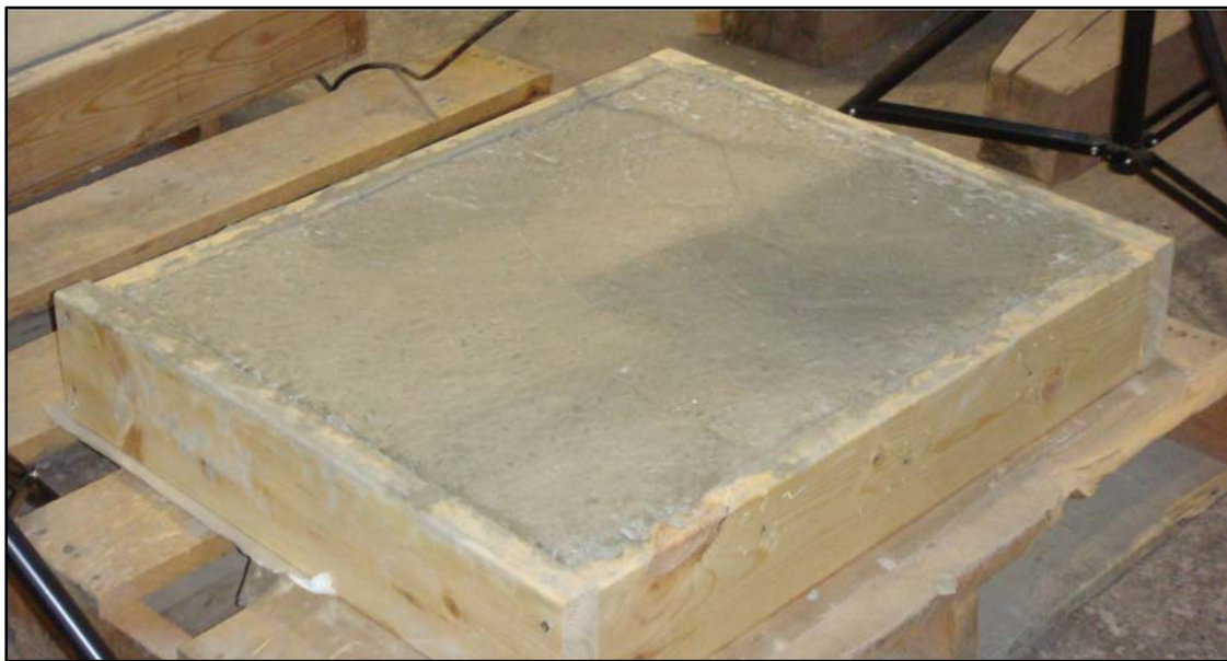
Figure 5.4 Concrete Slab II after it was cured.
