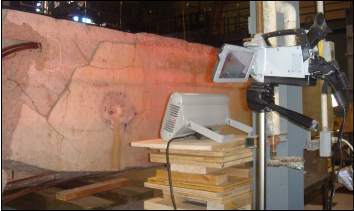
Figure C.7 Active infrared thermography test set-up at the location E4.
