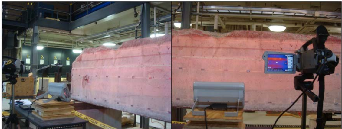
Figure C.8 Set-up for Active infrared thermography at location W4, where no delamination is evident.
