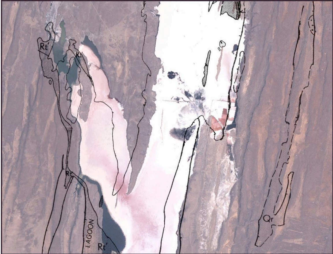
Figure 8: Mosaic of central portion of Lake Magadi using geologic map (Baker 1958), which has been simplified to a line drawing, and Landsat image (bands 1,2,3). Coordinate offset between the geologic map (black lines) and the Landsat image is clearly evident. Offsets range from 590-800 m and displacement azimuths vary between 70-122°.
