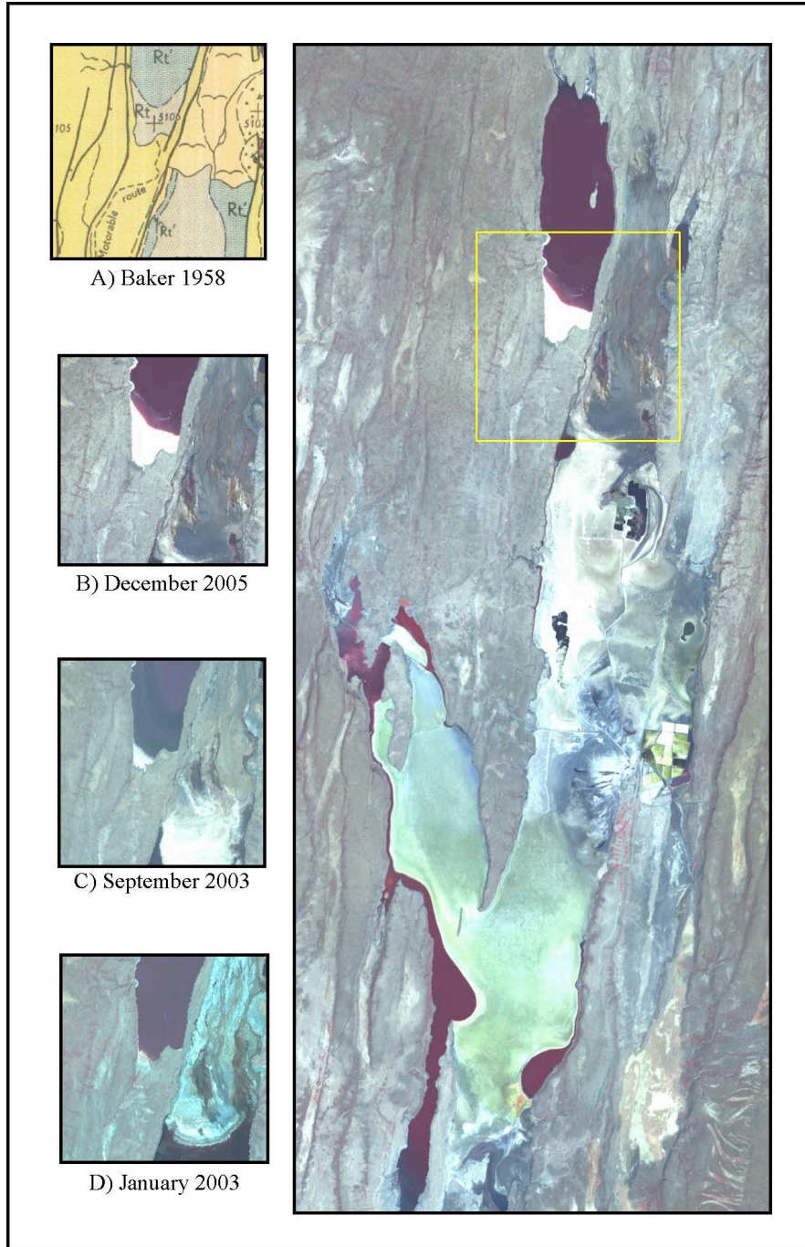
Figure 13: Comparison of exposed trona in the southern end of Little Magadi. Image on the right is a December 2005 ASTER image with the yellow box showing the area of interest as seen during different years on the left. A: Baker's 1958 Geologic Map B: December 2005, a known dry year. Note the large exposure of trona (bright white), which is probably exposed due to lower water levels. C, D: 2003 was a more normal year in terms of precipitation and the exposed trona is significantly less than in B. This clearly shows that the amount of trona exposed is the result of a dynamic system and will vary year to year.
