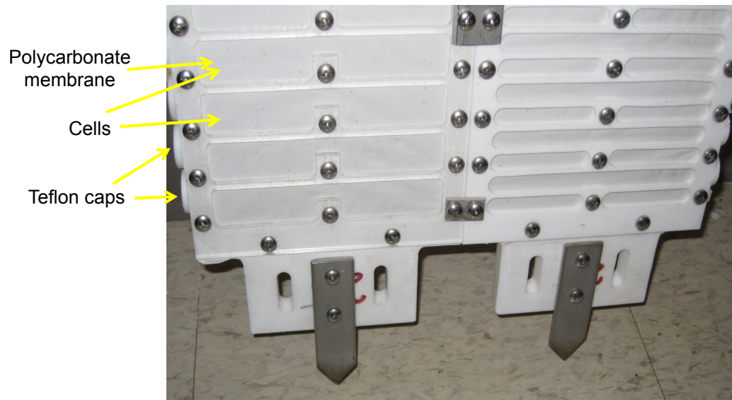
Figure 3.2: Modified Hesslein Sampler (peeper): Close-up of cells.
