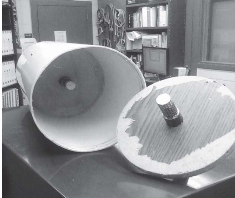
Figure 3.9: A picture showing the internal baffle, extended tubes, and perforated tubing used for one of the correlated experimental models.
