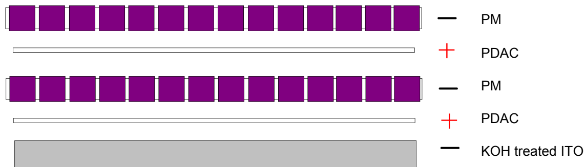
Figure 60. Layering process to create bR/PDAC multi-layered monolayer films.
