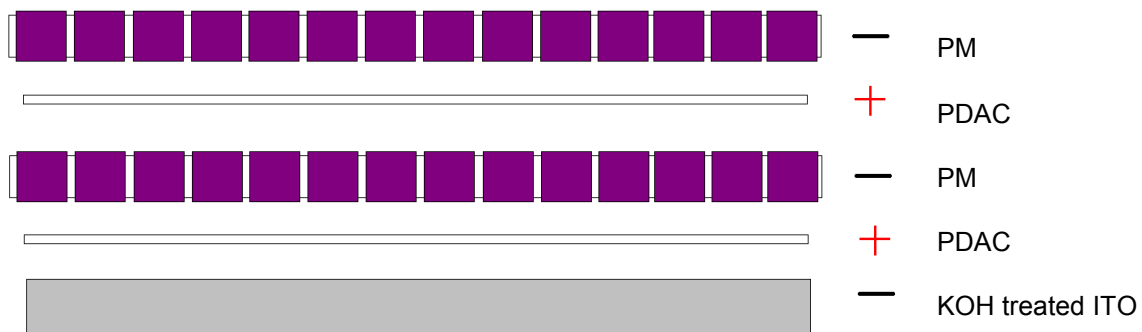
Figure 22. Schematic of bilayer I-SAM films constructed on negatively charged ITO with PDAC serving as the polycation and PM serving as the polyanion.
