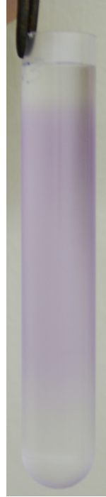
Figure 24. Sonicated PM in preformed linear sucrose gradient following ultracentrifugation.
