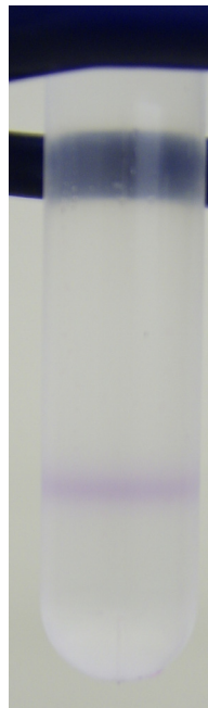
Figure 21. Post-centrifugation of PM in linear sucrose gradients. The PM band formed at a density of \sim 1.17 \text{ g mL}^{-1} .
