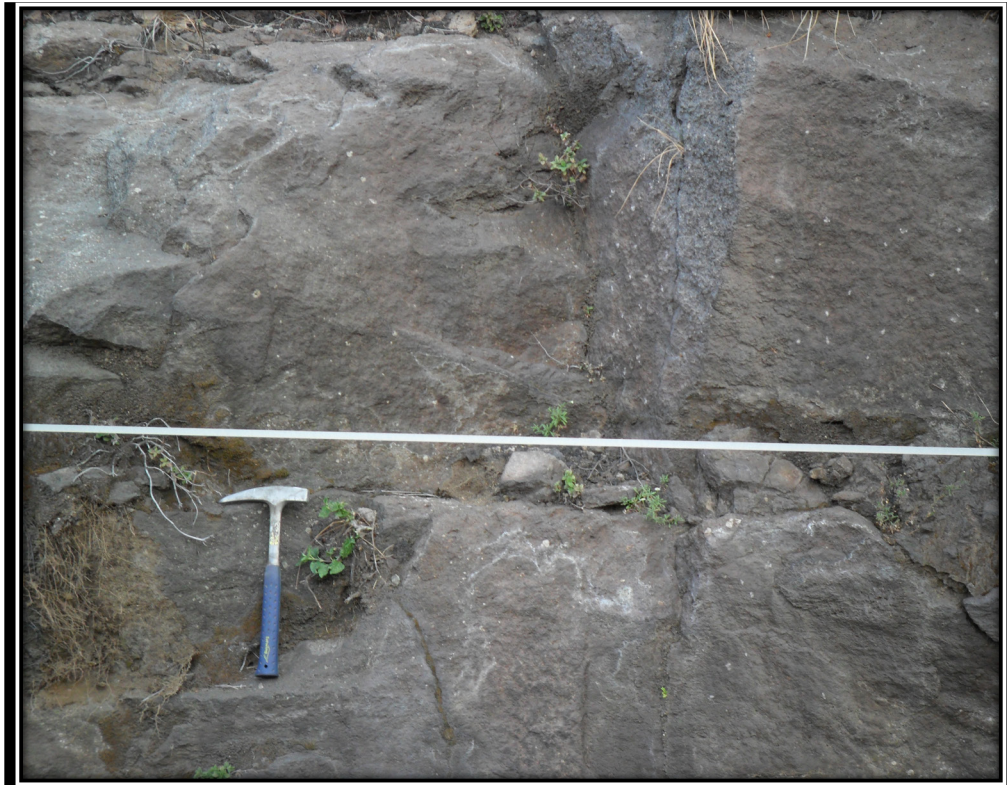
Figure 4.5: Lava outcrop, site A120, with surfaces slightly weathered with very small joint opening.
