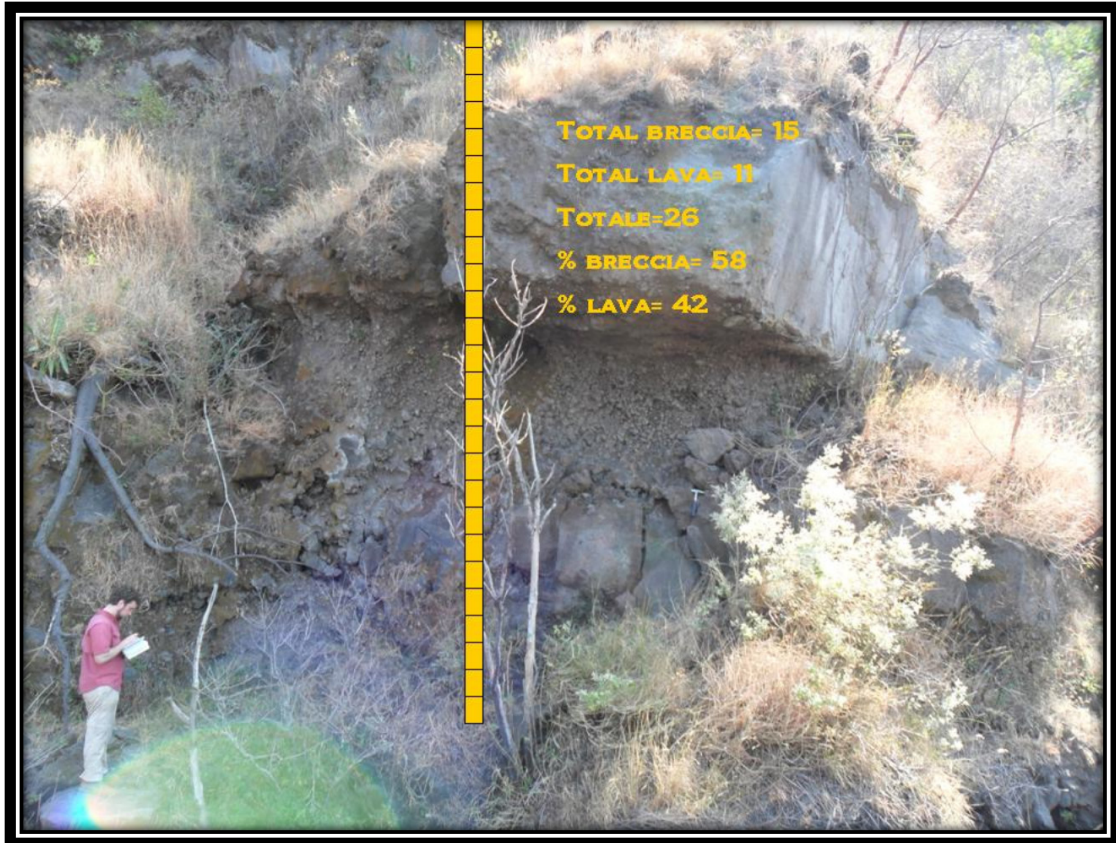
Figure 4.11: Image processing method to classify lithotechnical units. Site A08, which is classified as BRECCIA-LAVA unit. Lava range to 42% compared to breccia of 58%.
