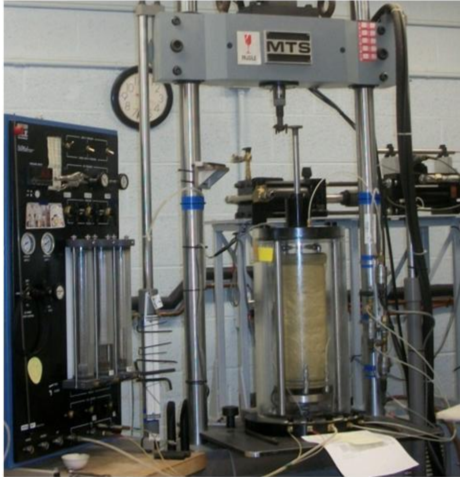
Figure 3.6: Triaxial Flexwall permeameter use to measure the coefficient of permeability of untreated OGM
