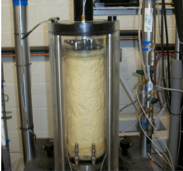
Figure 3. 7: Measuring the K of CTPB
