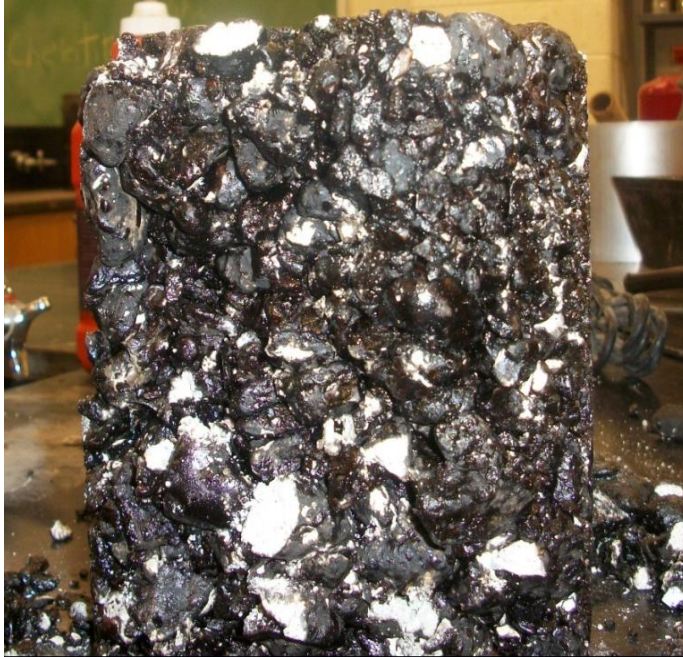
Figure 3. 9: ATPB samples disintegrating
