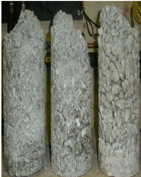
Figure 3. 8: CTPB samples after UCS testing
