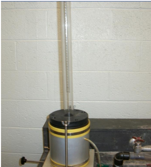
Figure 3. 10: Test apparatus used to measure the K of ATPB samples
