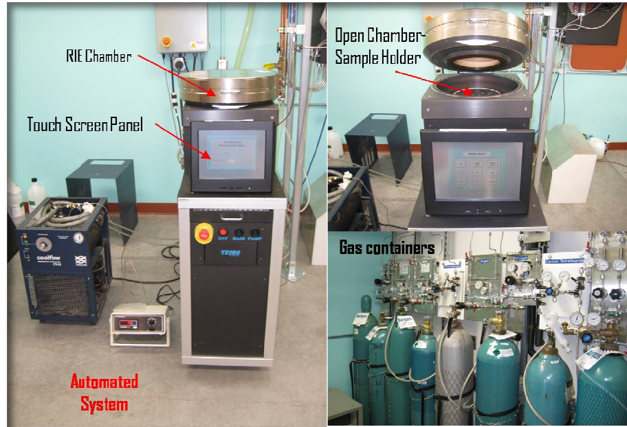
Figure 4.28: TRION ICP-RIE system, which was used for all the etch characterizations. The gas containers shown in the (c) are CF_4 , Nitrogen, Argon, CHF_3 , Oxygen, SF_6 etc.
