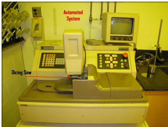
Figure 4.26: Automated Dicing System which was used for all the dicing purposes.
