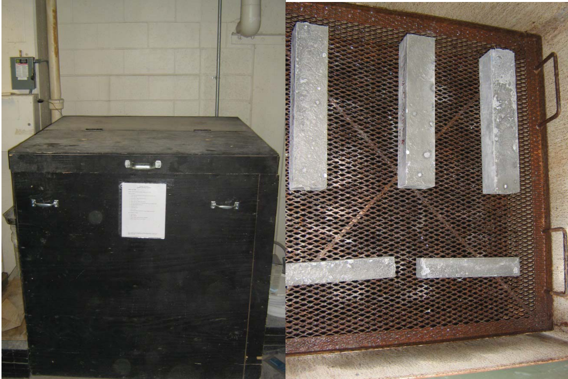
Figure 5.1: Curing chamber: external view (left) and internal view (Right)
