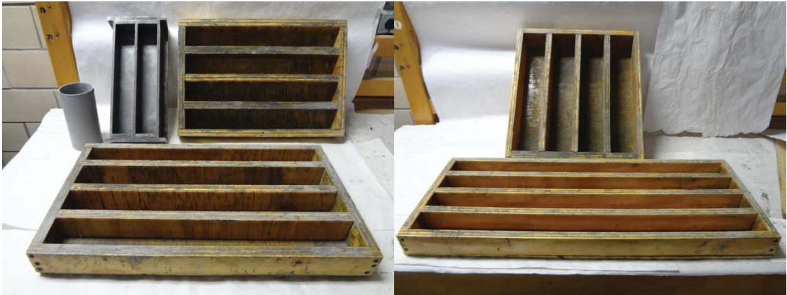
Figure 5.2: Molds: compression, 2580-4.5 prism, 2580-6.75 prism, 2580-9 prism, (left) , 5180-4.5 prism, 2600-13.25 prism (right)
