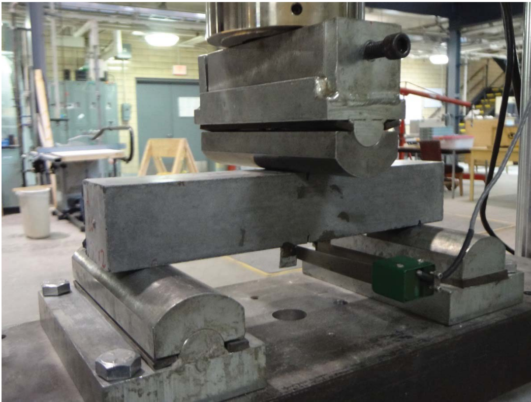
Figure 5.7: Fracture test setup
