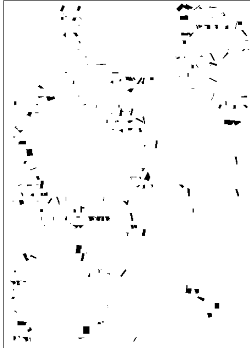
(d) Tensile forces within mastic at iterative steps = 500,000 (Maximum = 1.302 \times 10^{-1} )
