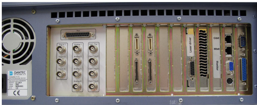
Figure 3.1 Dantec Dynamics FlowMap system hub.
