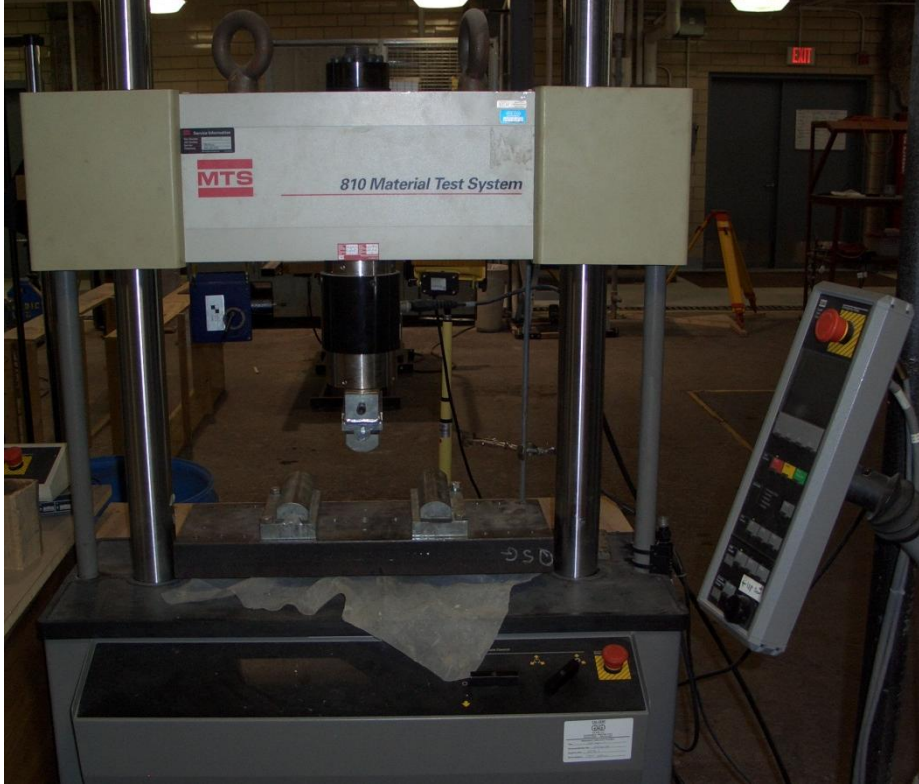
Figure 8: MTS Compression Machine
