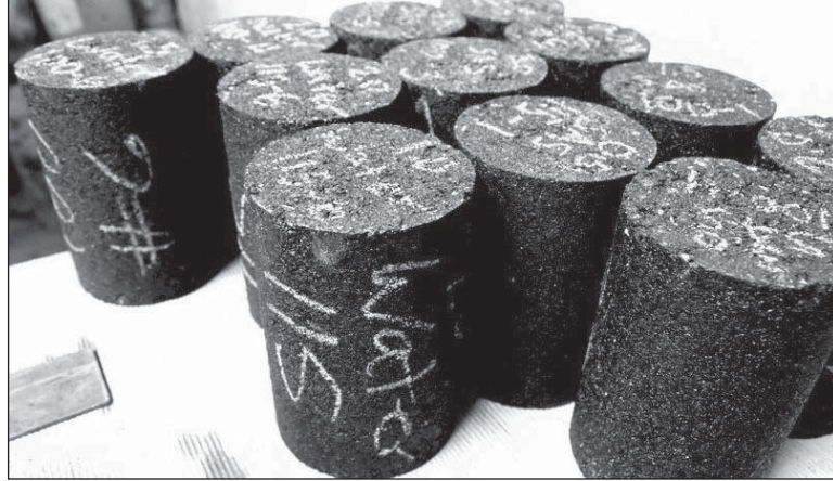
Figure 2.27 Warm Asphalt Mixture Produced using the Water Foaming Method
