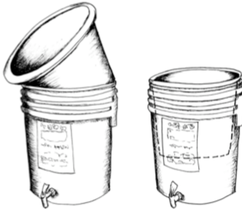
Figure 8: A sketch of the type of ceramic filter promoted by Potters for Peace (image courtesy of Linda Phillips)
