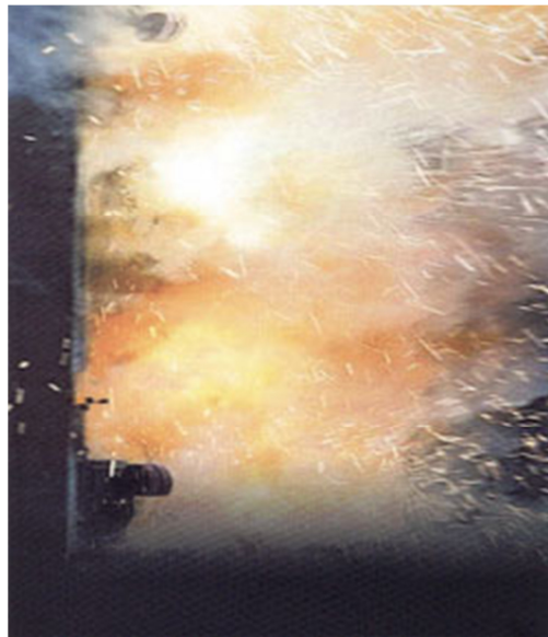
Figure 1.1: Lab demonstration of arc-flash explosion
