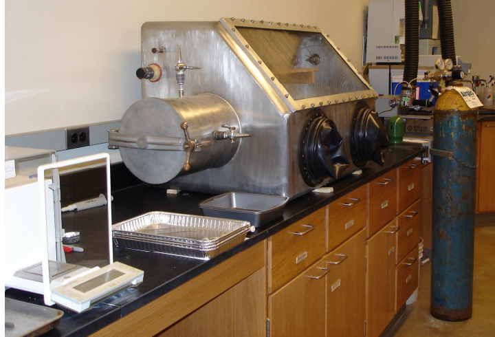
Figure 3. Reaction chamber used during the batch experiments.
